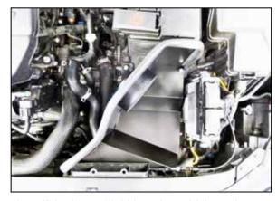
7. Install the heat shield into the vehicle and secure to the air filter housing mounting locations with the hardware provided.
