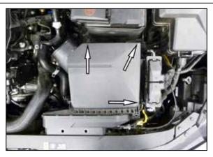
5. Remove the three bolts that secure the air filter housing and then remove the housing from the vehicle.
