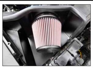
12. Install the K&N air filter onto the intake tube and secure with the provided hose clamp.
