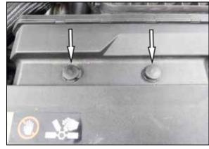
4. Raise the center of the push pin to release them and then remove the push pins from the vehicle.
