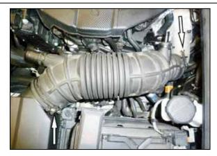
Loosen the hose clamps that secure the factory intake tube and then remove the tube from the vehicle.
