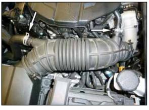
2. Release the spring clamps and then disconnect the CCV hose and BOV hose from the intake tube.
