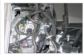
25. Install the provided crank case vent hose onto the 90° fitting in the K&N® intake tube and then attach the open end to the valve cover port.
