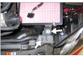
9. Remove the two bolts shown and then remove the front air box mounting bracket from the vehicle. NOTE: The bolt which secures the bracket to the core support will be reused in a later step.
