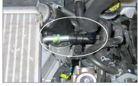
5. Rotate the crank case vent backwards to gain access to the green retaining clip. Using a small screw driver, release the locking tabs and then unhook the crank case vent from the valve cover port. Remove the green retaining clip from the valve cover port.
