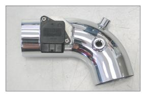
20. Install the mass air sensor into the  $K\&N^{\mbox{\scriptsize @}}$  intake tube and secure with the provided hardware.
