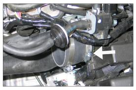
14.Install the provided silicone hose (084016) onto the turbo inlet tube and secure it with the provided hose clamp.
