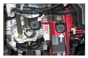
12. Remove the two air box mounting grommets
