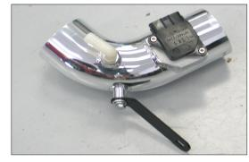
22. Install the tube mounting bracket (083130) onto the K&N® intake tube as shown.
