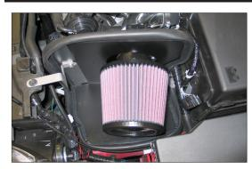
27. Install the K&N® air filter onto the intake tube and secure with the provided hose clamp. NOTE: Drycharger® air filter wrap; part # RX-4990DK is available to purchase separately. To learn more about Drycharger® filter wraps or look up color availability please visit http://www.knfilters.com®.
