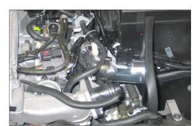
24. Install the K&N® intake tube assembly into the silicone hose at the turbo inlet pipe and align the bracket with the pop off valve mounting location. Secure the intake tube with the provided hose clamp and hardware.
