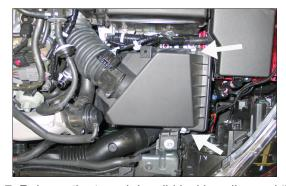
7. Release the two air box lid locking clips and then remove the air box lid from the vehicle.
