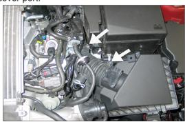
6. Loosen the two hose clamps which secure the intake tube to the air filter and turbo inlet tube.
