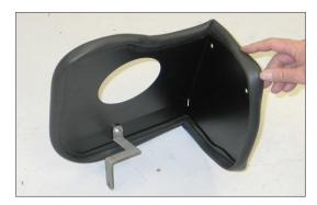
17. Install the heat shield mounting bracket (083131) onto the heat shield as shown using the provided hardware.
