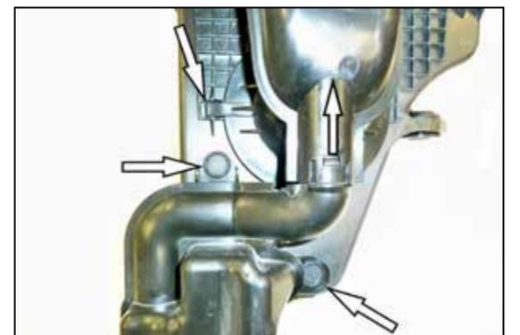
6. Remove the two push-pins that secure the fresh air duct to the air filter housing, release the locking tab and then rotate the duct counter clockwise to remove it from the air filter housing.
