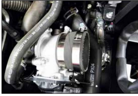
12. Install the provided coupler onto the throttle body and secure with the provided hose clamp.
