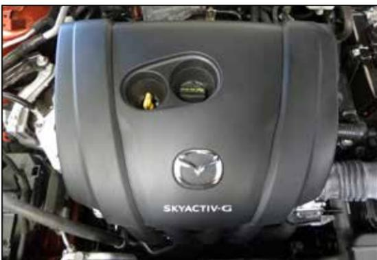
2. Pull straight up on the engine cover to remove it from the engine.
