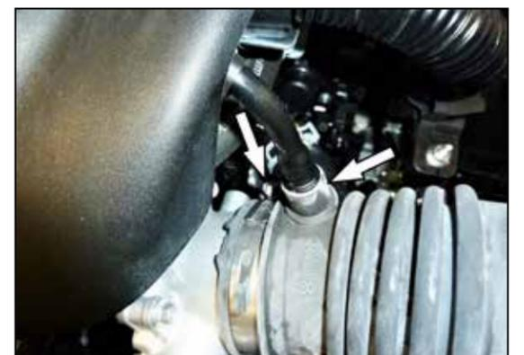
5. Loosen the hose clamp that secures the intake hose to the throttle body and then disconnect the CCV pipe from the intake hose. Lift the complete intake assembly up and remove it from the vehicle.
