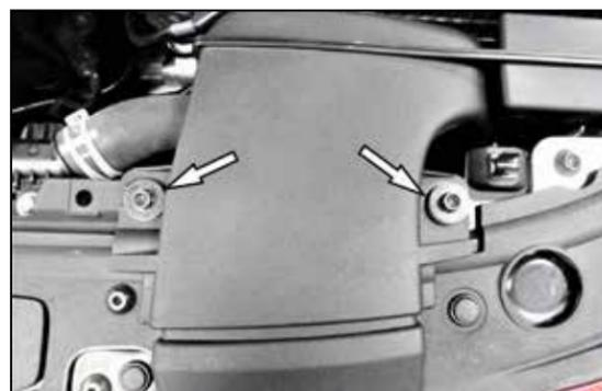
3. Remove the two bolts that secure the fresh air intake duct.
