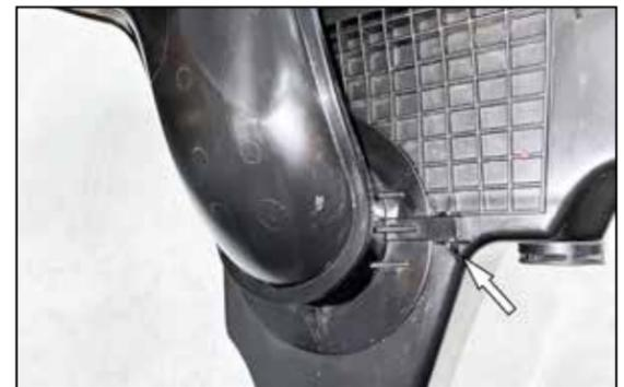
8. Release the tab that locks the fresh air duct onto the factory air filter housing, rotate the duct counterclockwise and then remove from the housing.
