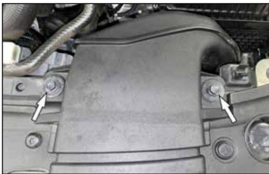
2. Remove the two bolts that secure the fresh air intake duct to the core support.
