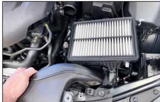
4. Lift the lower air filter housing up off the mounting posts and then remove the lower air filter housing from the vehicle.
