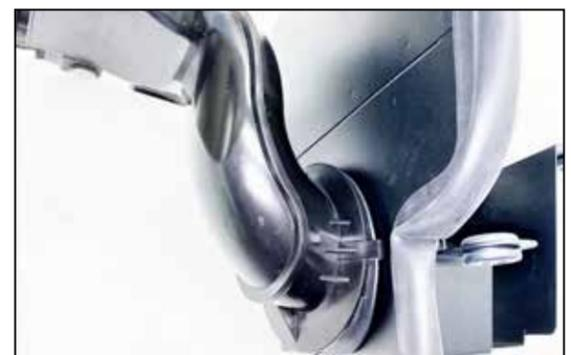
9. Install the fresh air intake duct into the K&N heatshield.
