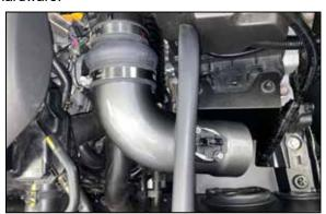
13. Install the intake tube assembly through the hole in the heatshield and then into the hump coupler and secure with the provided hose clamp.
