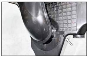
8. Release the tab that locks the fresh air duct onto the factory air filter housing, rotate the duct counterclockwise and then remove from the housing
