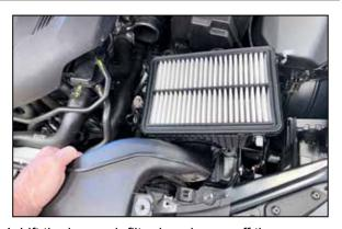
4. Lift the lower air filter housing up off the mounting posts and then remove the lower air filter housing from the vehicle.
