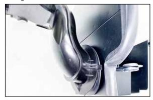
9. Install the fresh air intake duct into the K&N heatshield.
