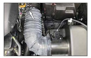
3. Loosen the hose clamp that secures the factory intake hose to the turbo inlet. Disconnect the mass air sensor and unhook the wiring harness from the air filter housing. Release the mounting clips and then remove the air filter housing lid and intake hose from the vehicle.
