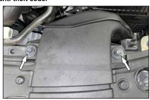
2. Remove the two bolts that secure the fresh air intake duct to the core support.
