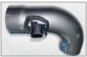
12. Remove the mass air sensor from the factory air filter housing and then install it into the K&N intake tube. Secure the sensor with the provided hardware.
