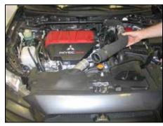
4. Remove the upper intercooler hose assembly from the vehicle.
