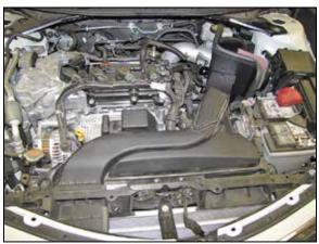
29. Install the fresh air intake scoop and secure with the factory hardware.
