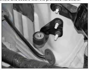
14. Install the remaining 1" tall rubber mounted stud onto the heat shield mounting bracket (26606) as shown.
