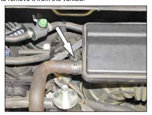
8. Release the spring clamp securing the crank case vent hose to the intake plenum and then disconnect the hose from the plenum.
