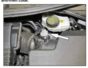
2. Disconnect the mass air sensor electrical connection and unhook the wiring harness from the air box.
