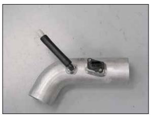
24. Install the crank case vent hose assembly onto the 90° fitting as shown.
