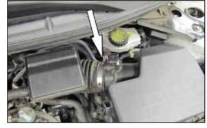
6. Loosen the hose clamp securing the intake hose to the air filter housing.
