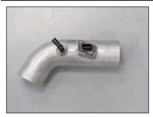
22. Install the 90° vent fitting into the K&N® intake tube as shown.
