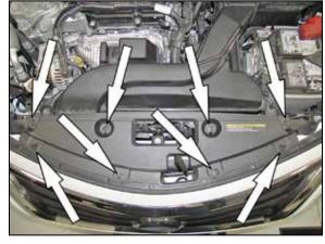
4. Pop up the eight plastic clips securing the core support cover and then remove the core support cover from the engine.
