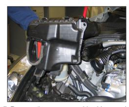
7. Remove the passenger side airbox as shown. NOTE: K&N Engineering, Inc., recommends that customers do not discard factory air intake.
