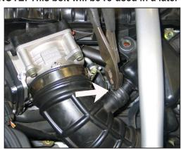
11. Release the spring clamp that retains the crankcase vent chamber. Then, disconnect the crankcase vent chamber from the stock intake tube.
