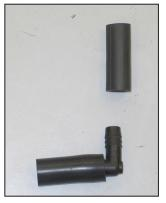
51. Install the two  $\frac{1}{2}$ " ID silicone hoses onto the provided 90° vent fitting as shown.
