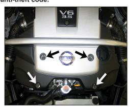
2. Remove the two front nuts and two rear bolts that secure the front engine cover. Then, remove the front engine cover from the engine.
