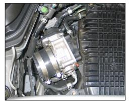
25. Install silicone hose (#08440) onto the throttle body and secure with the provided hose clamp as shown.
