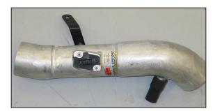
24. Install the mass air sensor into the K&N<sup>®</sup> intake tube and secure with the provided hardware.
