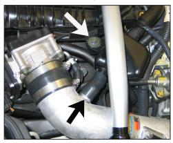
27. Install the crankcase vent chamber into the silicone hose attached to the vent tube of the  $K\&N^{\textcircled{\$}}$  intake tube. Secure the vent chamber with the bolt removed in step #10.
