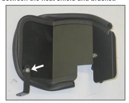
45. Install the provided heat shield mounting bracket (#010031) onto the top of the heat shield and secure using the provided hardware and spacer.
