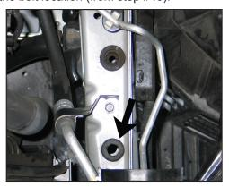
42. Install the nut insert into the airbox mounting grommet hole (shown).
