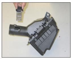
49. Remove the mass air sensor from the factory airbox as shown.
