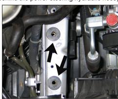
16. Install the two nut inserts into the factory airbox mounting grommet holes as shown.
