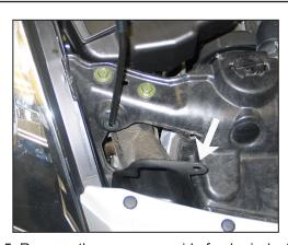
5. Remove the passenger side fresh air duct retaining clip. Slide the fresh air duct forward to disengage it from the passenger side airbox.
