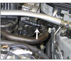
53. Connect the crankcase vent chamber into the 90° vent fitting assembly (installed in step #52).
