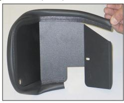
43. Install the provided edge trim onto the heat shield (#07367) as shown.
