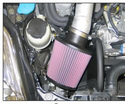
28. Install the K&N $^{\circledR}$  air filter and secure with the provided hose clamp. NOTE: Drycharger $^{\circledR}$  air filter wrap; part #
