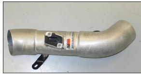
50. Install the mass air sensor into the K&N $^{\circledR}$  intake tube (#27540) and secure with the provided hardware.
