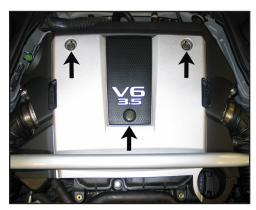
3. Remove the two nuts and one bolt that secure the rear engine cover. Then, remove the engine cover from the engine.
