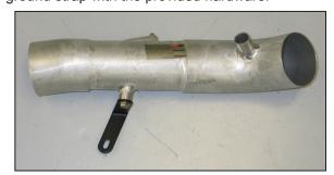
21. Install the tube mounting bracket (#26664) onto the intake tube (#27539) using the provided hardware as shown.
