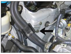
13. Remove the lower battery cable mounting bracket bolt shown.
