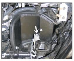
46. Install the heat shield assembly into the vehicle and align the lower bracket with the inserted nut, then align the upper bracket between the fan shroud and radiator. Secure the lower bracket with the provided hardware. Secure the upper bracket with the factory bolt removed in step #36.
