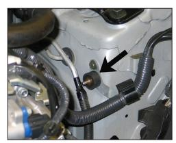
41. Install the provided rubber mounted stud into the bolt location (from step #40).
