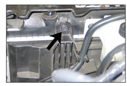
36. Remove the radiator cooling fan mounting bolt (shown).
