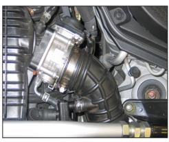
37. Loosen the hose clamp that secures the driver's side intake tube to the throttle body.
