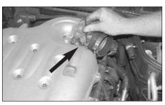
19. Install the provided silicone hose and hose clamps onto the throttle body and tighten.
