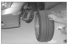
10. Raise the vehicle up and support it with jack stands, then, remove the front driver side tire as shown.
