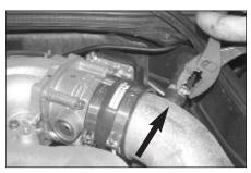
21. Reconnect the crank case vent hose as shown.
