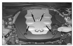
2. Remove the engine cover as shown.
