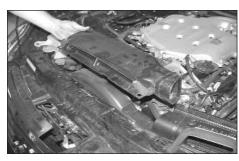
8. Disengage the two plastic rivets, then, remove the stock air inlet duct as shown.
