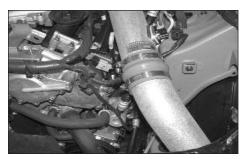
27. Slide the silicone hose over the short ram tube as shown.
