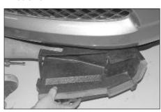
15. Remove the styrofoam/plastic block off panel as shown.
