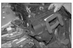
9. Pull firmly upwards to release the air cleaner base from the factory grommets, then remove the air cleaner base as shown. NOTE: K&N Engineering, Inc., recommends that customers do not discard factory air intake.
