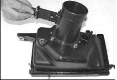
17. Loosen and remove the two screws to remove the mass air sensor from the stock air cleaner lid as shown.
