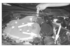
4. Loosen the hose clamps at the throttle body and at the mass air sensor, then, loosen and remove the bolt that secures the resonator to the intake manifold.
