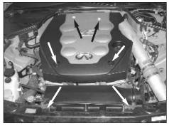
33. Reinstall the engine cover and the air inlet duct as shown.
