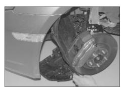
11. Remove the nine bolts and six plastic rivets, then, lower the inner fender valance down as shown.
