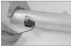
18. Insert the mass air sensor from step 17 into the K&N® Typhoon® short ram tube using the provided hardware.
