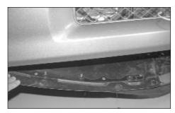
13. Remove the three bolts that secure the lower splash guard, then lower the splash guard down as shown.
