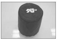
29. Install the provided K&N® Drycharger® onto the K&N air filter as shown. NOTE: The Drychargers water repellent properties will last up to two years. See the parts list to reorder a new Drycharger if necessary.
