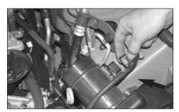
6. Disconnect the mass air sensor electrical connection as shown.
