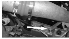
28. Secure the bracket to the rubber mounted stud using the provided hardware as shown, but do not tighten completely at this time.
