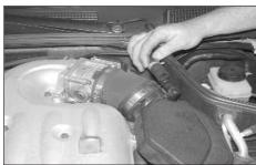
3. Disconnect the crank case vent hose as shown.
