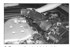
5. Remove the stock intake tube as shown.
