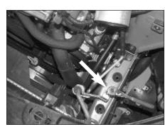
22. Remove the bolt that secures the a/c hard line bracket to the inner fender as shown.
