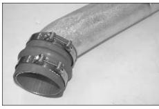
25. Slide the silicone hose and hose clamps onto the K&N® Typhoon® cold air tube as shown.
