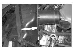
7. Unclip the air cleaner lid, then, loosen and remove the single bolt that secures the air cleaner lid to the fender. Rotate the air cleaner lid, then, unclip the mass air sensor electrical connection to remove the air cleaner lid as shown
