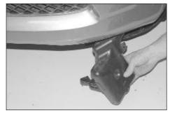
12. Remove the two bolts that secure the resonator to the inner fender, then, remove the resonator as shown.
