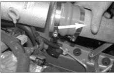
26. Install the K&N® Typhoon® cold air tube into the vehicle and line up the bracket with the rubber mounted stud as shown.
