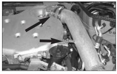
20. Install the K&N<sup>®</sup> Typhoon<sup>®</sup> short ram tube into the silicone hose at the throttle body, then, secure the bracket to the threaded hole on the manifold using the bolt removed in step 4.
