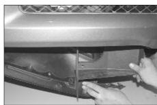
16. Remove the plastic cover from the styrofoam block off panel from step 15 and reinsert the plastic cover onto the radiator core support and secure it with the plastic rivets.
