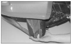
30. Install the K&N® air filter onto the K&N Typhoon® cold air tube as shown.
