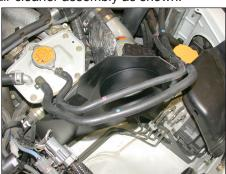
20. Install the stock coolant clips onto the two tabs on the heat shield, then clip the coolant lines onto the clips as shown.
