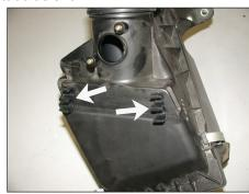
19. Remove the stock coolant clips from the stock air cleaner assembly as shown.
