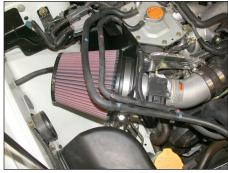
24. Install the K&N® air filter and secure using the provided hose clamp as shown.
