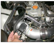
23. Reroute the mass air sensor electrical connection behind the heat shield and between the heat deflector plate and reconnect as shown.
