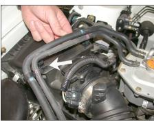
3. Unclip the coolant lines from the top of the air cleaner as shown.
