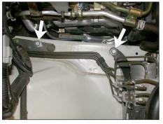
14. Reinstall the original air cleaner mounting bolts as shown above.
