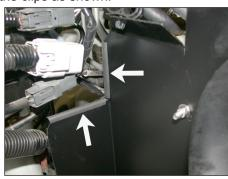
21. Cut the provided edge trim to size and place onto the heat shield as shown.
