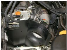
16. Install the complete air cleaner assembly into the vehicle and slide the intake tube into the silicone hose as shown above.
