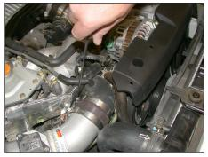
18. Tighten the hose clamp on the K&N® intake tube as shown.
