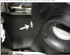
17. Secure the heat shield to the "Z" bracket using the provided hardware as shown.
