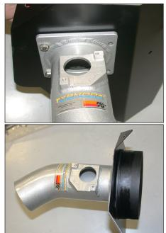
10. Assemble the tube, heat shield, filter adapter, and the remaining gasket using two of the provided hex bolts as shown above.
