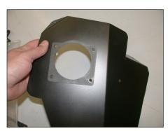
9. Install one of the provided gaskets onto the back of the heat shield as shown.
