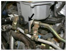
13. Install the provided "Z" bracket onto the coolant reservoir using the original nut removed in step 14.
