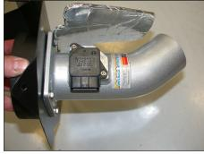
15. Install the mass air sensor into the K&N® intake tube using the provided screws as shown above.
