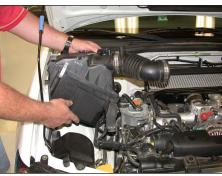
6. Remove the complete air cleaner assembly as shown.
