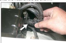
22. Unclip the wire harness from the inner fender bracket as some slack will be needed to reroute the mass air sensor electrical connection.
