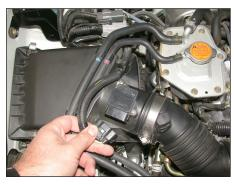
2. Disconnect the mass air sensor electrical connection as shown.
