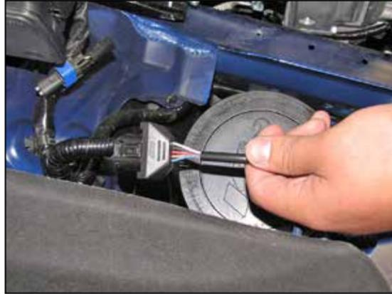
13. Connect the mass air sensor extension harness provided into the factory mass air sensor connector and then connect the open end to the mass air sensor.
