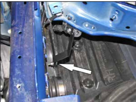
11. Install the tube mounting bracket (064327) into the factory intake tube mounting location using the provided hardware.
