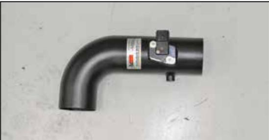
9. Install the mass air sensor into the K&N® intake tube and secure with the provided hardware.
