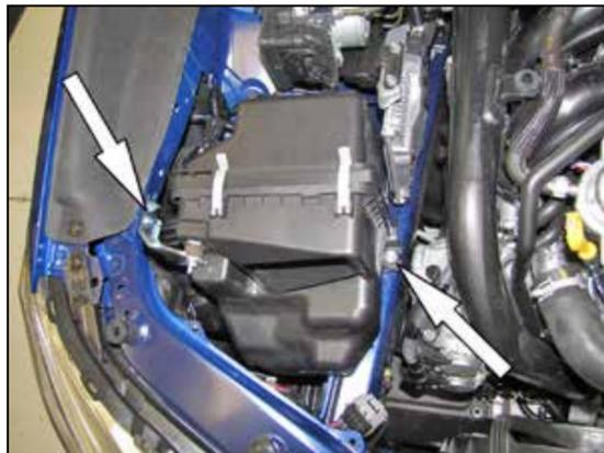
3. Remove the two nuts and one bolt securing the front half of the air filter housing to the vehicle.
