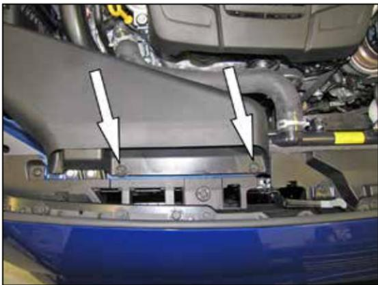
2. Remove the two clips shown securing the fresh air intake scoop and then remove the fresh air intake scoop.
