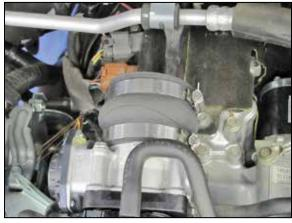
18. Install one of the provided coupler hoses onto the throttle body and secure with the provided hose clamp.
