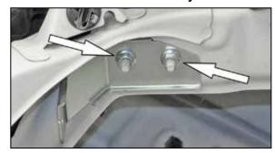
9. Remove the two nuts that secure the air filter housing bracket onto the inner fender.
