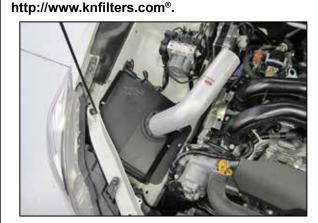
17. Install the intake tube/heat shield assembly into the engine compartment as shown and connect the mass air sensor connection, then secure the heat shield with the provided hardware and factory nuts from step 8.
