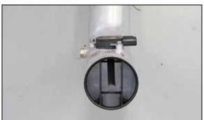
14. Place four drops of the provided super glue onto the lip of the provided air grid and then install the air grid into the K&N® intake tube as shown.
