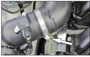
5. Loosen the hose clamp securing the intake tube to the air filter housing and then remove the intake tube from the vehicle.
