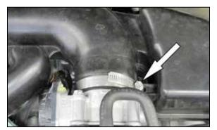
4. Loosen the hose clamp securing the intake tube to the throttle body.
