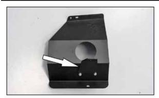
10. Install the tube mounting bracket (064326) onto the heat shield as shown.
