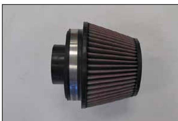
9. Install the K&N® air filter onto the provided filter adapter and secure with the provided hose clamp.
