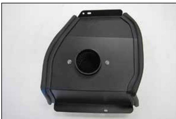
10. Install the filter assembly into the heat shield assembly and secure with the provided hardware.
