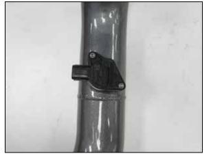
13. Remove the mass air sensor from the factory housing and install it into the K&N intake tube using the provided hardware.
