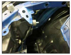
11. Install the provided vibration damper onto the factory air filter housing mounting location using the factory nut.
