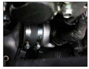
15. Install the provided coupler onto the turbo inlet along with the provided hose clamps. Do not tighten the clamps.
