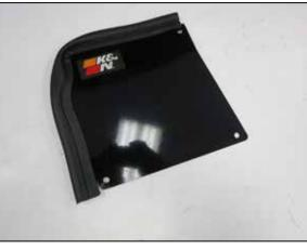
24. Install the remaining 15" edge trim onto the lid as shown. Install the K&N badge and secure with the backing plate.
