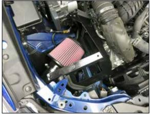
22. Install the mounting posts into the factory air filter housing mounting locations on the inner fender, then install the K&N heat shield onto the poste
