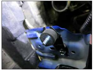
12. Install the provided vibration damper onto the factory intake tube mounting location using the factory nut.
