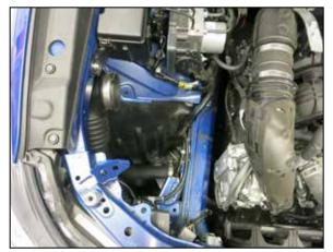
7. Remove the remaining air filter housing half from the engine compartment.
