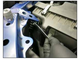
5. Remove the nut the secures the vibration damper to the core support. This nut will be reused in a later step.
