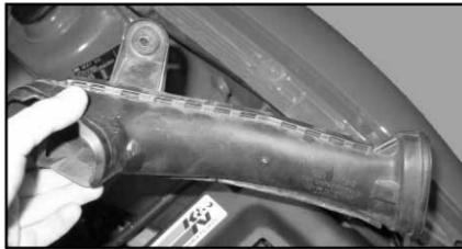
8. Remove the nut that secures the air inlet duct and remove the air inlet duct from the vehicle as shown.
