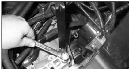
10. Mount the "Z" bracket onto the gear box mount using its original bolt. (do not fully tighten yet!)
