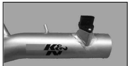
14. Mount the MAS onto the new intake tube using the two M5 bolts supplied. **NOTE:** Before installing, inspect the inside of the tube for any debris, then clean the inside out with water and a towel.
