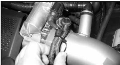
25. Zip tie the crank case vent switch connection to the throttle control connection using the provided cable tie as shown.
