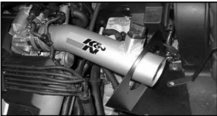
19. Align the tube and the bracket for best clearance. Now remove the heat shield assembly, keeping the tube and bracket in place.
