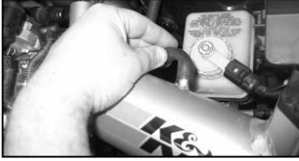
22. Fit the small breather onto the intake tube.
