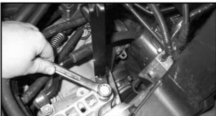
20. Now firmly tighten the gear box mounting bolt and the M6 bolt on the intake tube.
