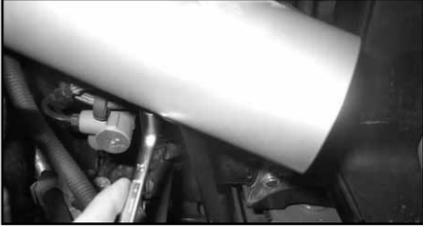
17. Fit the intake tube onto the bracket using the hardware supplied.
