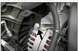
19. Install the tube mounting bracket onto the alternator and secure with the bolt removed in the previous step.
