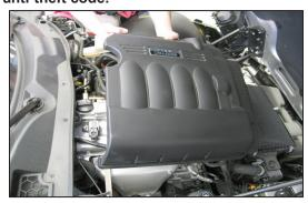
2. Lift firmly on the engine cover to dislodge it from the mounting grommets and then remove the engine cover assembly.
