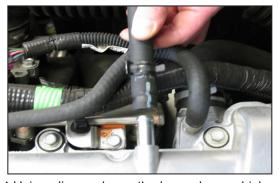
4.Using pliers, release the hose clamp which secures the crankcase vent hose to the valve cover and then remove the crankcase vent hose from the valve cover as shown.
