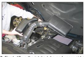
7. Firmly lift up the intake tube and upper airbox to release it from the mounting grommets and then remove the assembly from the vehicle.
