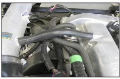
21. Install the supplied crankcase vent hose onto the valve cover and onto the intake tube as shown. NOTE: Some trimming of the hose may be necessary.
