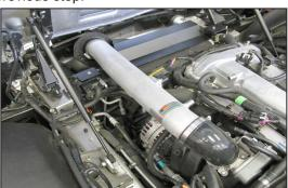
20. Install the K&N® intake tube assembly into the silicone hose at the throttle body and align with the mounting bracket installed in the previous step. Secure the tube with the hose clamp and hardware provided.
