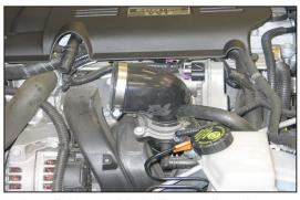
16. Install the provided silicone elbow hose onto the throttle body and secure with provided hose clamp.
