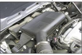
6. Release the six upper airbox mounting clips.
