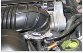
5. Loosen the hose clamp which secures the stock intake tube to the throttle body.
