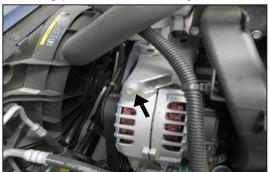
18. Remove the upper alternator mounting bolt. **NOTE: This bolt will be reused in the next step.**
