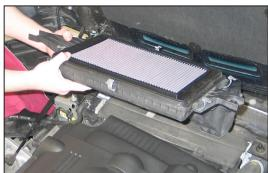
9. Pull up firmly to release the lower airbox housing from the mounting grommets and then remove the lower airbox from the vehicle.
