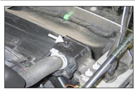
10. Remove the right lower airbox mounting studs shown from the bracket.
