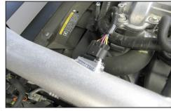
22. Connect the mass air sensor electrical connection.
