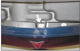
8. Remove the front lower airbox mounting bolt shown.
