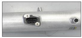
13. Install the mass air sensor into the K&N® intake tube and secure with the provided screws.
