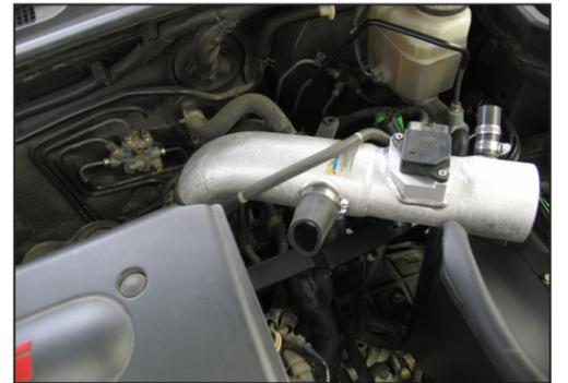
21. Install the K&N intake tube into the silicone (084016) hose on the throttle body; and align with the intake tube mounting bracket which was installed in step 13.
