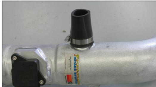
17. Install the provided silicone hose (084074) onto the K&N intake tube and secure with the provided hose clamp.
