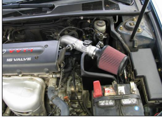
27. Reconnect the vehicle's negative battery cable. Check to ensure all hose clamps and fittings are properly tightened and positioned correctly before starting the vehicle.
