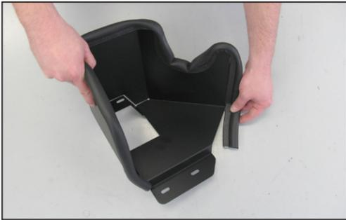
10. Install the provided edge trim onto the heat shield as shown in the photograph.
