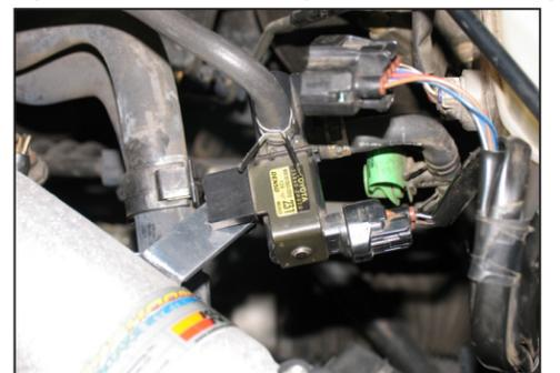
24. Install the pulse width modulated (PWM) switching valve into the grommet on the welded bracket on the intake tube as shown in the photograph.
