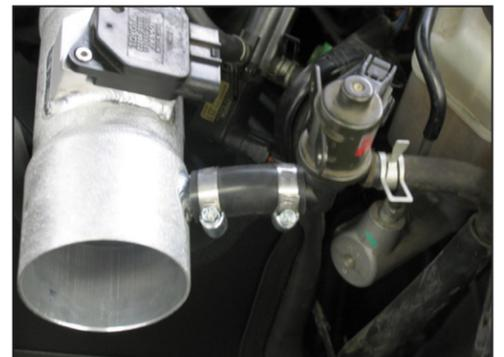
23. On vehicles equipped with an "EVAP canister closed valve", install the "EVAP canister closed valve" into the silicone hose which was installed in step 19; secure with the provided hose clamp.
