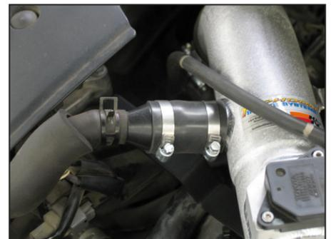
22. Install the crank case vent hose/chamber into the silicone hose installed onto the K&N intake tube in step 19; secure with the provided hose clamp.
