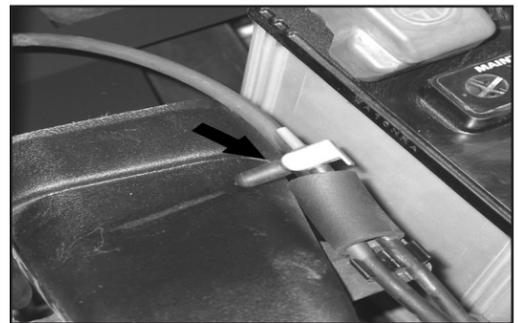
27. Install one vacuum cap plug onto the the factory "T" fitting as shown in the photograph.
