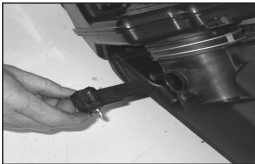
21. Remove the two screws that secure the mass air sensor to the stock intake tube. Remove the mass air sensor as shown in the photograph.
