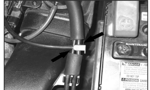
8. Disconnect the two vacuum lines from the factory "T" fitting.
