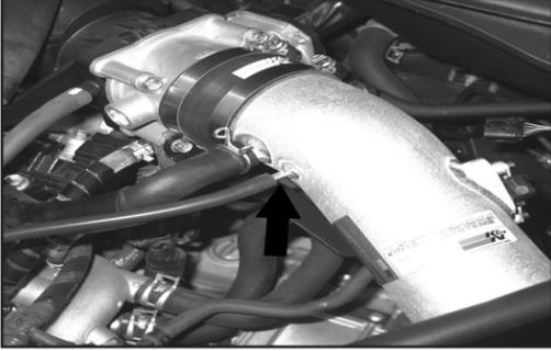
30. Install the supplied vacuum hose to the K&N® Intake Tube.
