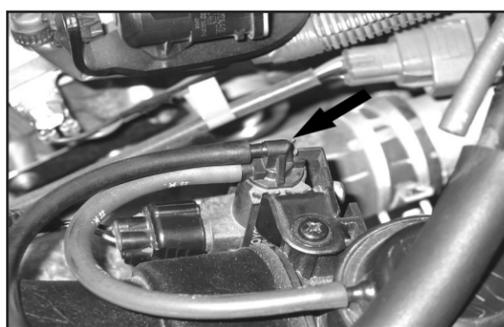
7. Disconnect the two vacuum lines from the "Vacuum switching valve."
