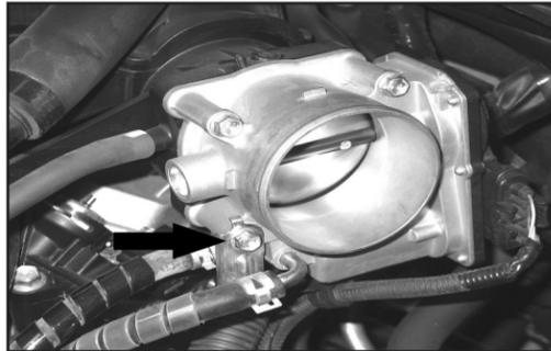
18. Remove the front lower throttle body mounting bolt.
