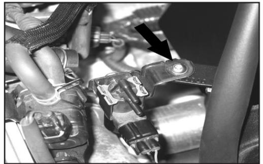
24. Secure the "vacuum switching valve" to the bracket installed onto the heat shield installed in step #16.
