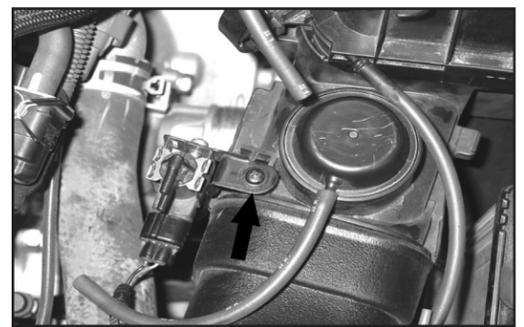
9. Remove the screw securing the "Vacuum switching valve" to the stock fresh air duct. Place the "Vacuum switching valve" in a position that will allow ample clearance to work around.
