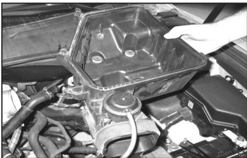
13. Remove the lower air box from the vehicle.
