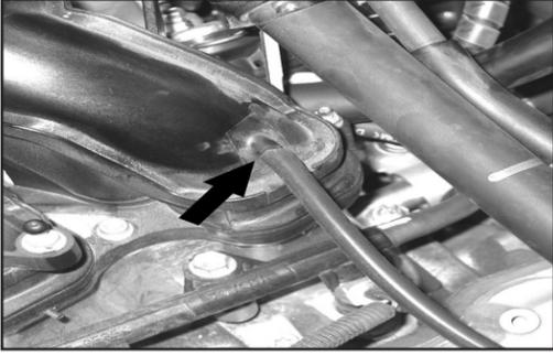
29. Connect the open end of the vacuum line installed in the previous step to the intake manifold plenum connection.
