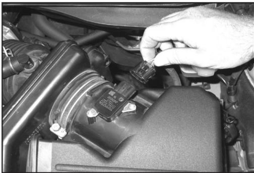
2. Disconnect the mass sensor electrical connection by depressing the center tab and gently pulling the harness away from the mass air sensor. Release the two wiring harness clips from the air box lid.
