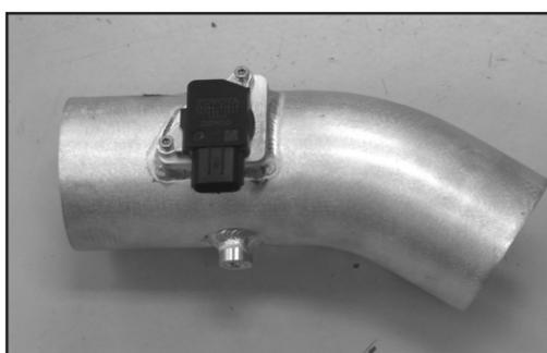
22. Install the mass air sensor removed in the previous step into the K&N intake tube and secure with the provided hardware.
