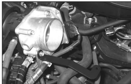
19. Install the intake tube mounting bracket (06485) onto the throttle body and secure with the bolt removed in the previous step.
