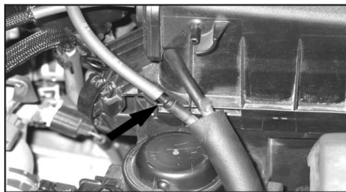
6. Disconnect the intake tube plenum vacuum line.
