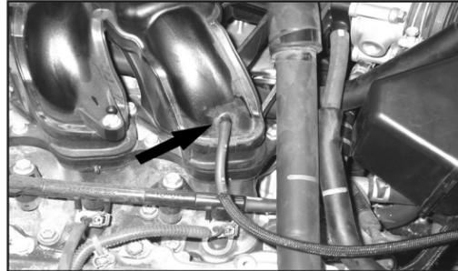
4. Disconnect the vacuum line from the intake manifold plenum connection.
