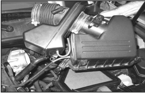
11. Release the clamps that secure the upper air box. Remove the upper air box and intake tube assembly.
