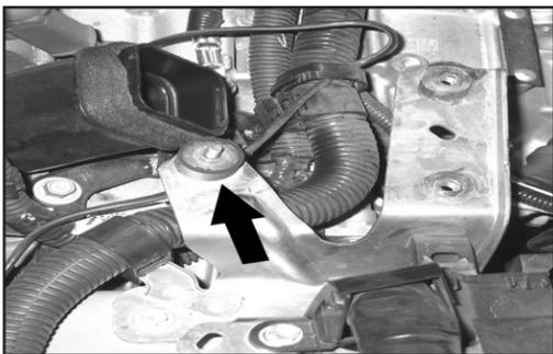
14. Install the rubber mounted stud onto the air box mounting bracket in the forward mounting hole location as shown in the photograph.
