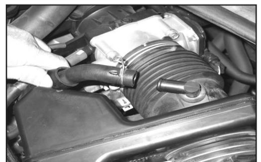
10. Release the clamp that secures the crank case vent hose to the stock intake tube and remove the crank case vent hose as shown. Loosen the clamp that secures the stock intake tube to the throttle body.
