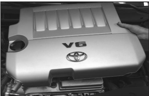
3. Gently pull the engine cover upward to release it from the mounting grommets. Once released, Remove engine cover from the vehicle and set aside.
