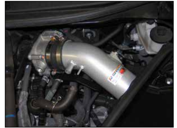
32. Install the K&N® intake tube into the silicone hose at the throttle body and align with the tube mounting bracket. Align the tube and bracket for proper fit and then secure with the provided hardware and hose clamp.
