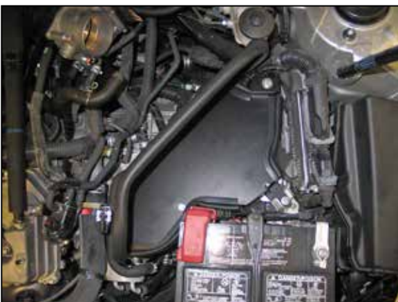
26. Set the heat shield into position and secure with the provided hardware.
