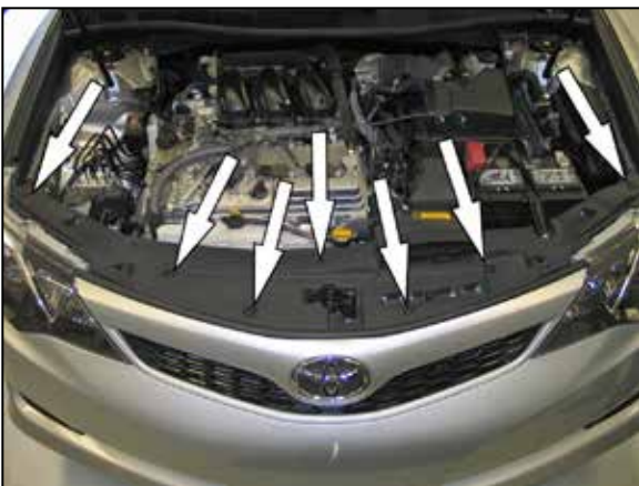
11. Remove the 7 clips securing the upper valance and then remove the upper valance from the vehicle.
