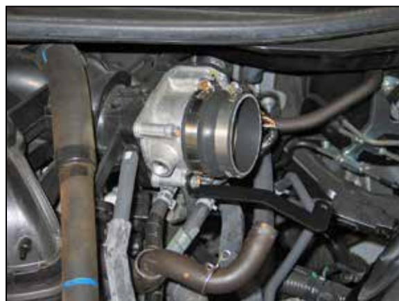
29. Install the silicone hose #084031 onto the throttle body and secure with the provided hose clamp.
