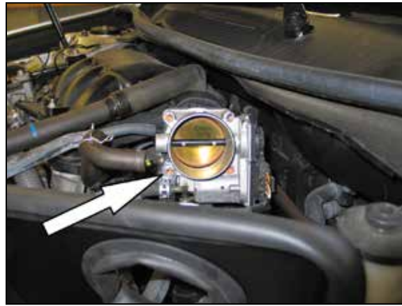
27. Remove the front lower throttle body mounting bolt shown. NOTE: This bolt will be reused in the next step.
