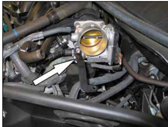
28. Install the tube mounting bracket (06485) onto the throttle body securing with the factory bolt removed in the previous step. NOTE: Do not completely tighten at this time.
