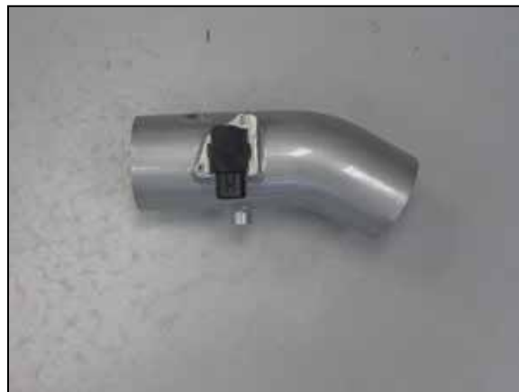
31. Install the mass air sensor into the K&N® intake tube and secure with the provided hardware.
