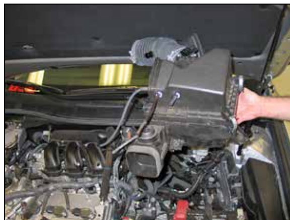
15. Remove the air box from the vehicle. NOTE: K&N Engineering, Inc., recommends that customers do not discard factory air intake.
