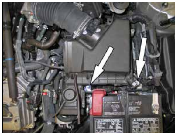
14. Remove the two bolts shown securing the air box.
