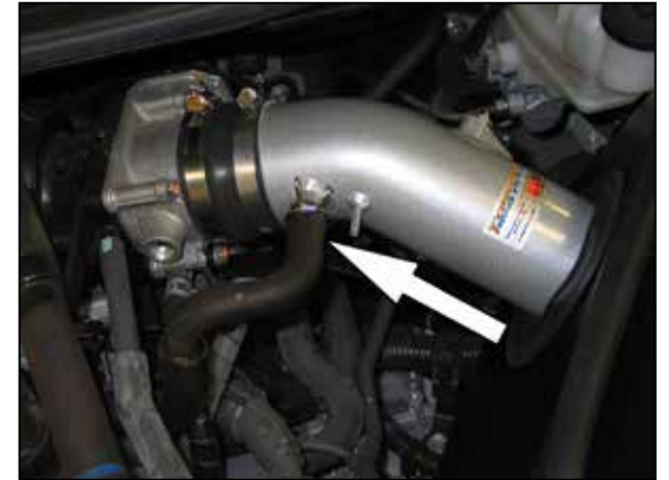
33. Connect the crank case vent hose to the K&N® intake tube and secure with the factory clamp.
