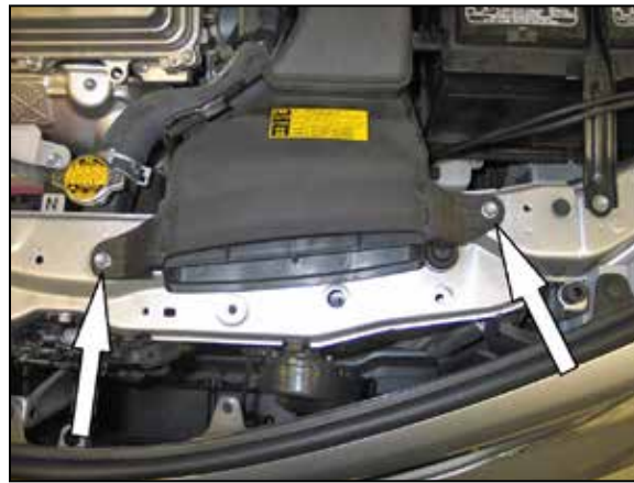
13. Remove the two bolts securing the fresh air duct and then remove the fresh air duct from the vehicle.
