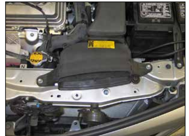
34. Reinstall the fresh air intake scoop and secure with the factory hardware.
