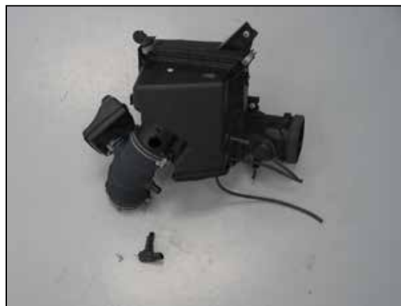
30. Remove the two screws securing the mass air sensor and then remove the mass air sensor from the factory air box.
