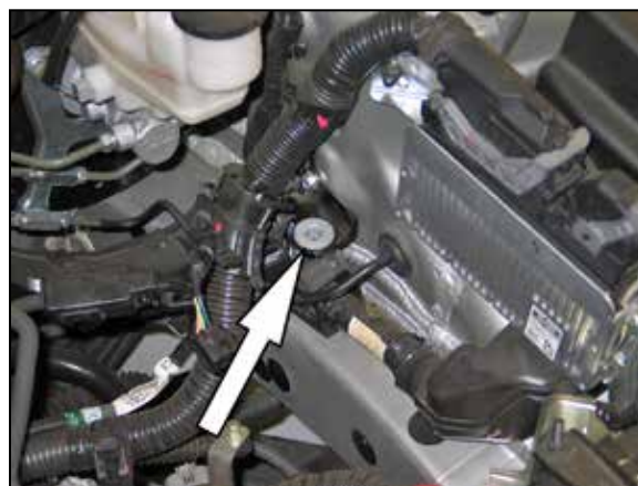
16. Remove the air box mounting grommet shown.
