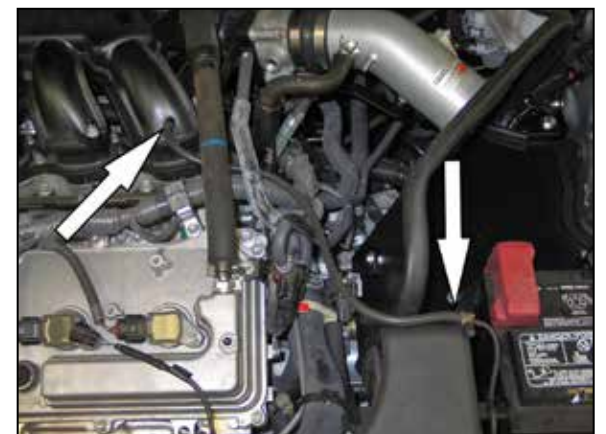
36. Install the provided longer vacuum hose to the vacuum TEE and install the open end onto the intake plenum.
