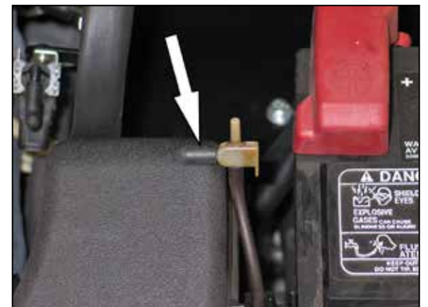
35. Install the provided vacuum plug onto the vacuum TEE.
