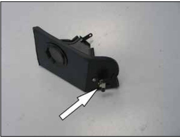
24. Secure the vacuum switching valve to the "L" bracket installed onto the heat shield as shown and then install the provided vacuum caps.
