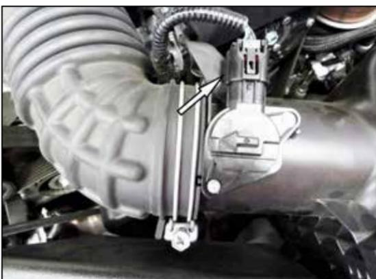
2. Disconnect the mass air sensor electrical connection and unhook the wiring harness from the air box.
