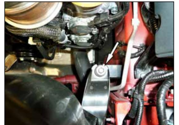
5. Remove the remaining air box mounting bolt then lift up the air box assembly and remove it from the vehicle. **NOTE: This bolt will be reused in a later step.**
