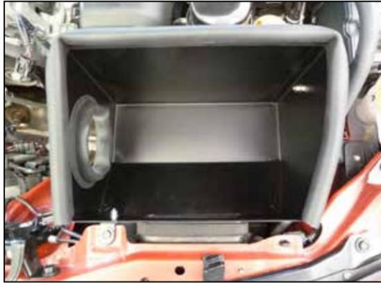
12. Set the heat shield into position on the core support and secure with the factory air box mounting bolts and to the previously install bracket with the hardware provided.
