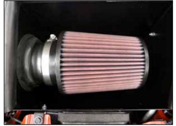
16. Install the K&N air filter onto the K&N intake tube and secure with the provided hose clamp.
