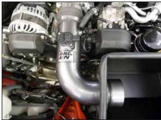
14. Install the tube through the heat shield. Rotate the tube down and install it into the silicone hose on the throttle body. Secure the tube with the provided hose clamp. **NOTE: The tube is a tight fit through the opening, take care so as not to damage the edge trim.**
