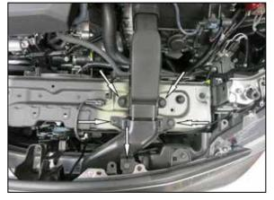
3. Remove the four plastic pins that secure the fresh air intake duct sections and then remove both sections of the fresh air duct.
