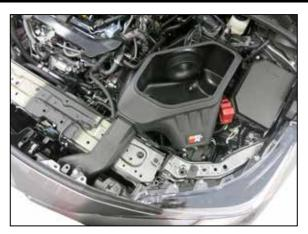
14. Set the K&N air filter housing into position, insert the duct into the air filter housing and then install the housing so the mounting studs insert into the factory housing mounting grommets.
