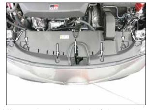
2. Remove the seven plastic pins that secure the radiator valence and then remove the valence from the vehicle.
