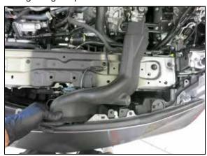
13. Feed the K&N fresh air duct over the core support down in behind the grill opening and then secure with the provided bolt. **NOTE: releasing the hood latch allows for easier access while installing the duct behind the grill.**
