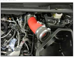
17. Install the tube assembly onto the turbo inlet by sliding the coupler onto the turbo, then align the tube and coupler with the filter adapter, adjust the tube and couplers for best fit and then secure all the hose clamps.
