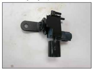
11. Remove the vacuum switch from the factory air filter housing and then secure the provided "L" bracket to the switch using the factory mounting bolt.
