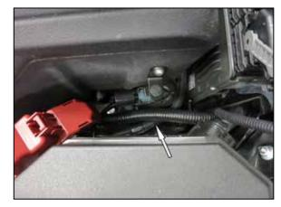
15. Reconnect the vacuum switch electrical connection.
