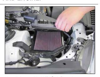
7. Install the provided K&N® air filter; do not secure the upper air box lid at this time.
