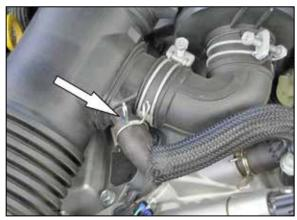
3. Release the spring clip securing the crank case breather hose to the factory intake tube and disconnect the crank case breather from the factory intake tube.
