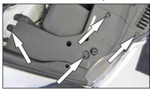
5. Remove the four clips securing the cover panel to the core support and inner fender, and then remove the panel from the vehicle.
