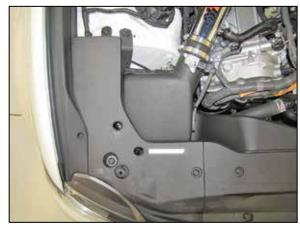
12. Reinstall the cover over the air box and secure with the four factory retaining clips.
