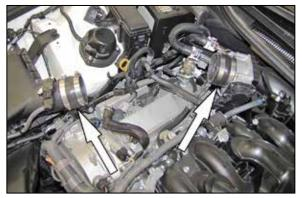
9. Install the provided coupling hoses (084031) onto the throttle body and air box as shown securing with the provided hose clamps
