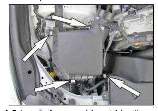
6. Release the four upper air box retaining clips and then remove the factory air filter.
