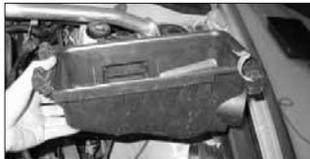
11. Remove the air box base as shown.
