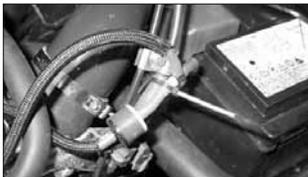
22b. **2005-later & compressor models:** Fit the vacuum hose onto the throttle cable using a tie wrap supplied.
