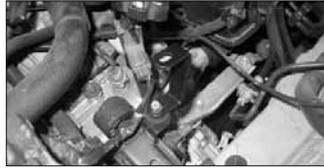
25. Install the "C" bracket to the rubber mounted stud using a waved washer and nylock nut supplied, but do not tighten completely.
