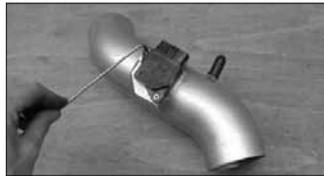
28. Install the mass air sensor into the adapter on the Typhoon intake tube and secure with the provided hardware
