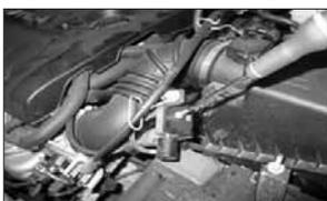
4. Remove the stock bracket from the vacuum switching valve as shown.
