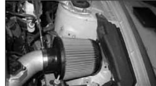
33. Install the Filter onto the tube and secure with the provided hose clamp as shown. Now firmly tighten all hose clamps and hardware connections!
