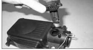
27. Remove the screws from the mass air sensor, then, remove the mass air sensor from the air box as shown.
