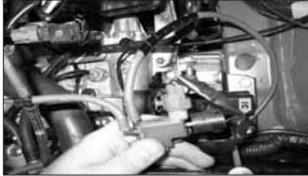
20. If fitted disconnect the two vacuum hoses from the vacuum switching valve as shown.
