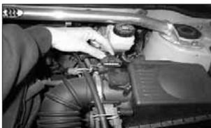
2. Disconnect the mass air sensor electrical connection as shown.
