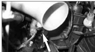
31. Align the Typhoon tube with the "C" bracket and secure with the M6 bolt and wave washer supplied. Don't fully tighten yet!
