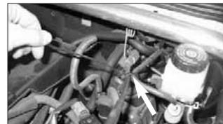
36. Secure the throttle cable to the brake line using the plastic cable tie supplied. **Do not fully tighten the cable tie, allow a little slack for the throttle cable!**
