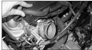
29. Install the silicone step hose and hose clamps supplied onto the throttle body as shown. Do not fully tighten yet!
