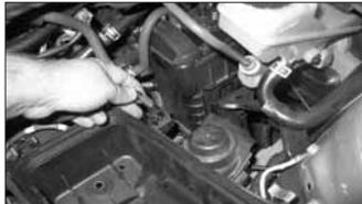
10. Unclip the wire harness from the air box base as shown.
