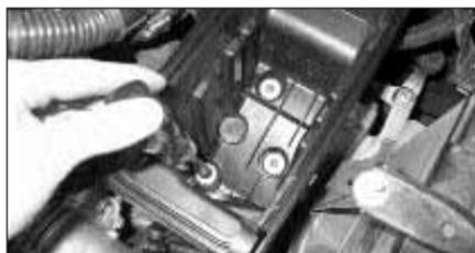
9. Remove the filter and undo the three bolts at the bottom of the air box base.
