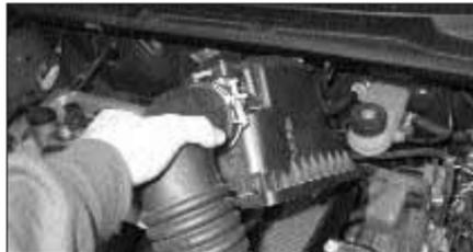
8. Unclip and remove the air box lid together with the intake hose.
