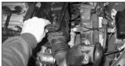
10. Unbolt the intake snorkel and remove the complete air box base from the vehicle.
