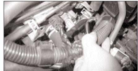
12. Unhook the wiring loom to give more clearance to the MAS connector lead.
