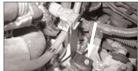
14. Fit the purge valve onto the L-bracket.
