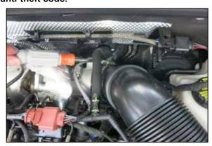
2. Loosen the hose clamp that secures the stock intake tube to the turbo inlet.
