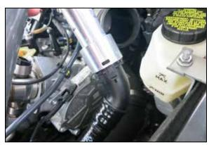
15. Connect the BOV hose to the fitting on the K&N intake tube.
