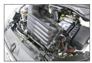
6. Remove the factory air filter housing from the vehicle.
