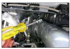
16. Insert the intake tube through the heat shield and into the coupler at the turbo, adjust for best fit and secure with the provided hose clamp.
