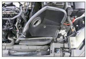
13. Set the heat shield into the vehicle so the mounting studs insert into the mounting grommets.
