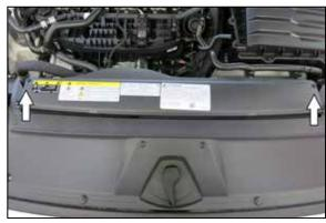
5. Remove the two screws that secure the fresh air inlet and then remove the fresh air inlet from the vehicle.
