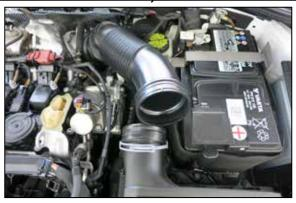
3. Release the spring clamp that secures the stock intake tube to the air filter housing and disconnect the tube from the housing.
