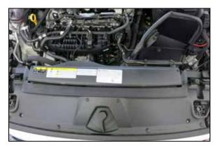
14. Reinstall the fresh air inlet and secure with the factory hardware.
