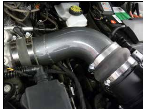
14. Install the K&N intake tube into the couplers, align for best fit and then secure with the provided hose clamps.
