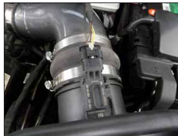
15. Reconnect the mass air sensor electrical connection.
