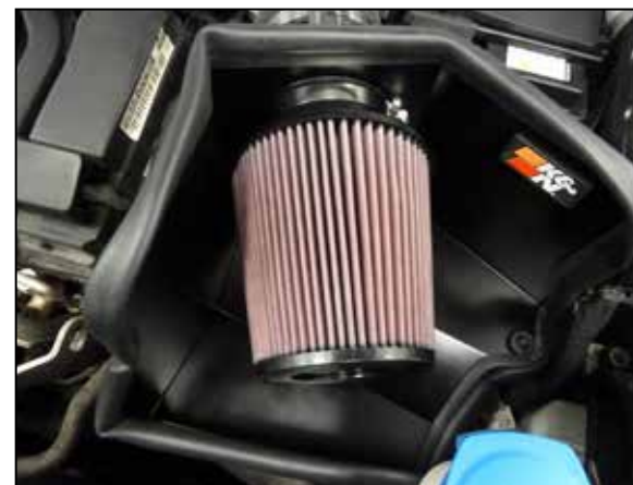
16. Install the K&N air filter and secure with the provided hose clamp.
