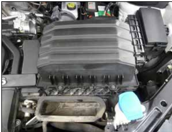
4. Pull the air filter housing straight up to dislodge it from the mounting grommets and remove it from the vehicle.
