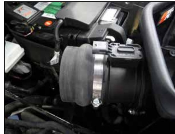
13. Install the provided hump coupler onto the mass air sensor and secure with the provided hose clamp.
