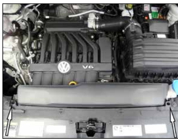
2. Remove the two screws securing the fresh air duct and then remove the duct from the engine compartment.
