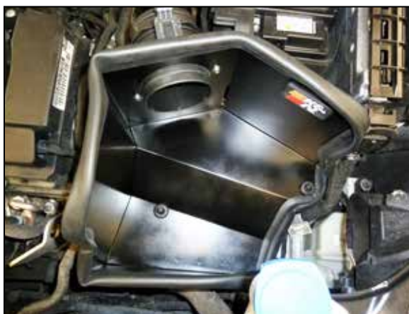
11. Set the heat shield assembly into the position on the factory mounting studs.
