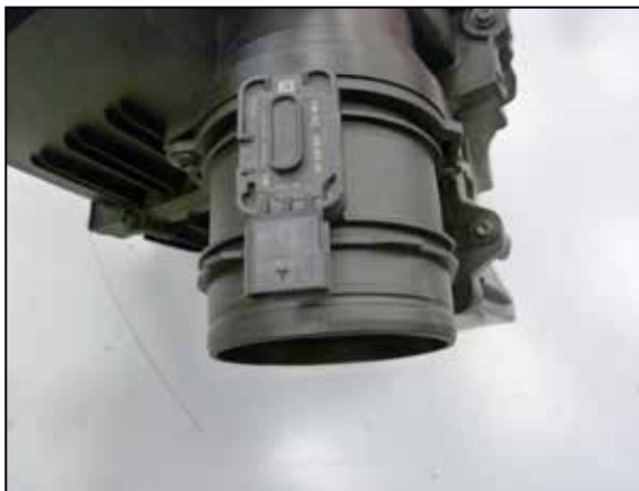
5. Remove the screws that secure the mass air sensor to the air filter housing and then remove the mass air sensor from the air filter housing.
