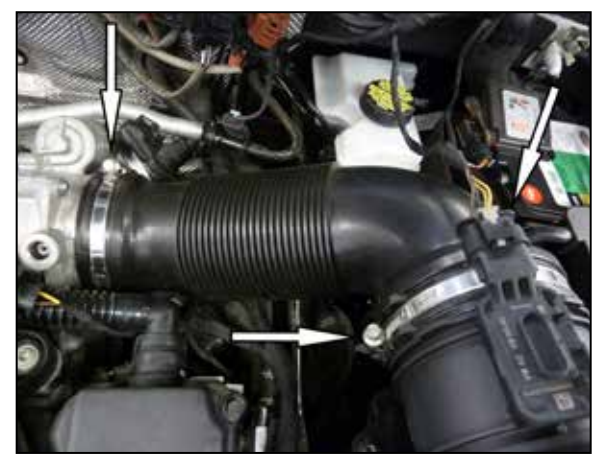
3. Loosen the hose clamps that secure the factory intake tube and remove the tube from the vehicle. Disconnect the mass air sensor electrical connection.
