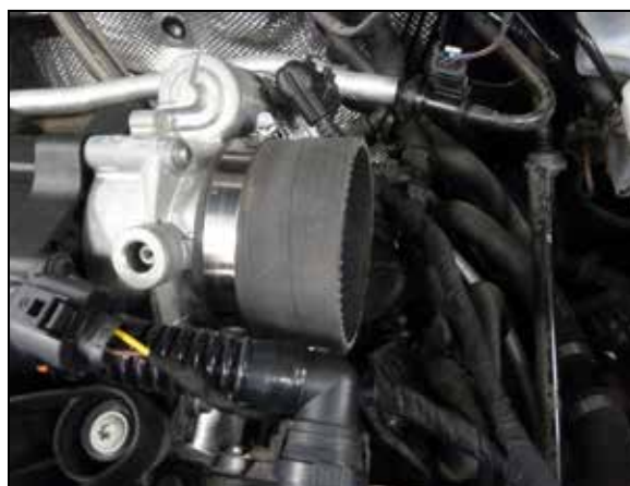
12. Install the provided coupler onto the throttle body and secure with the provided hose clamp.
