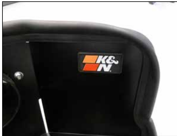
9. Install the K&N badge onto the heat shield.
