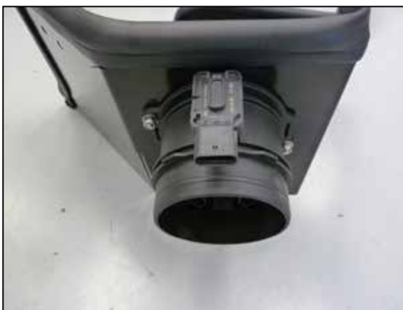
8. Install the mass air sensor onto the heat shield using the provided hardware.
