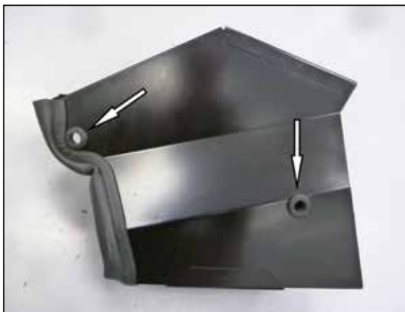
7. Install the two provided grommets into the heat shield as shown.
