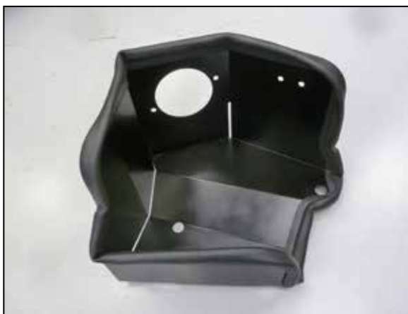
6. Install the provided edge trim onto the heat shield as shown. NOTE: it will be necessary to trim the edge trim.
