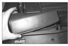
4. Unclip and remove the intake snorkel lid as shown.
