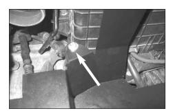
15. Fit the heat shield to the air box support bracket using a M6 bolt and a flat M6 washer supplied.
