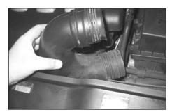
6. Unclip and remove the air box feed pipe from the vehicle as shown
