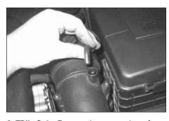
3. TDI's Only: Remove the vacuum hose from the top or the side of the air box as shown.
