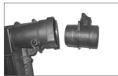
9. Remove the MAS from the airbox as shown.
