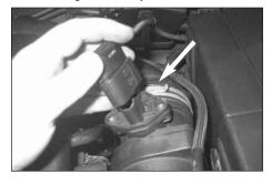
2. Disconnect the Mass Air Sensor (MAS) electrical connection as shown.
