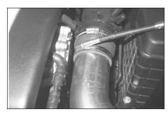
18. Fit the intake tube into the sleeve using the hose clamp supplied. Do not fully tighten at this moment.
