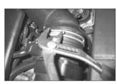
7. Unclip the intake hose clamp from the MAS as shown.
