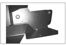
13. Fit the rubber grommets into the 2 holes of the heat shield as shown.
