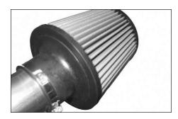
16. Mount the filter onto the intake tube using the hose clamp supplied.
