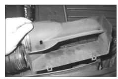
5. Unclip and remove the intake snorkel as shown.
