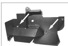
12. Install the 2 heat shields using the 2 short M6 Allen bolts, and M6 washers supplied.
