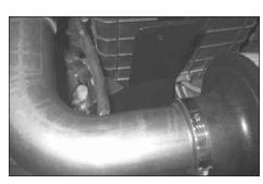
21.TDI's Only: Fit the vent plug onto the original vacuum hose and extend it using the small vacuum hose supplied. Fit the vacuum hose to the intake tube as shown
