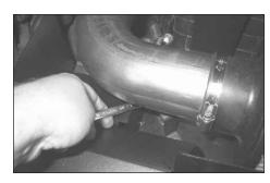
20. Align the Typhoon tube and filter for the best clearance and tighten all bolts and clamps.
