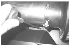
19. Fit the bracket to the heat shield using the large M6 bolt, M6 washer supplied. Do not fully tighten yet!
