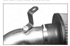
17. Fit the bracket to the intake tube as shown using the M6 Nylock nut, waved washer and flat metal washer supplied. Don't fully tighten yet!
