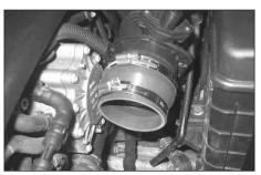
11. Fit the sleeve supplied to the MAS using the hose clamps supplied. 1.9 TDi & 1.8TFSi use the small sleeve.
