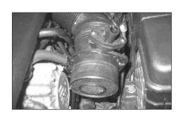
10. Refit the MAS to the engines intake using its original hose clamp as shown.
