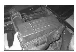
8. Unbolt and remove the air box assembly from the vehicle as shown.
