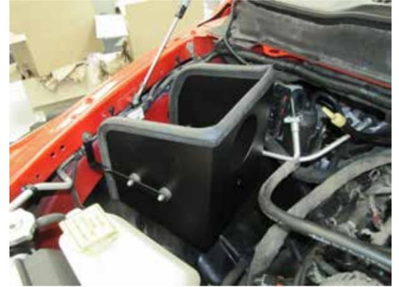
19. Install the heat shield assembly into the vehicle and secure to the bracket previously installed, to the inner fender and rubber mounted stud.
