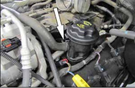
8. Release the spring clamp and then disconnect the crank case vent hose from the breather port.
