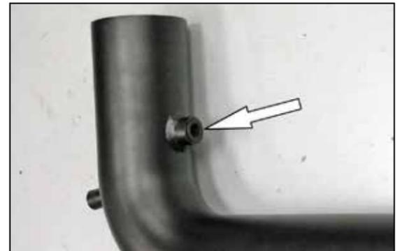
22. Install the silicone hose into the inlet air temperature sensor mount as shown.
