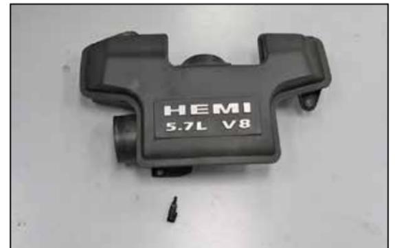
23. Remove the inlet temperature sensor from the intake plenum and then remove the O-ring from the sensor.
