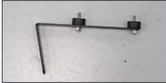
13. Install the two of the rubber mounted studs onto the provided bracket (070050) and secure with the provided hardware.
