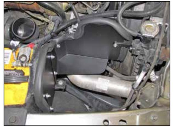
17. Set the heat shield onto the air box mounting tabs so that the inserts engage with the mounts, align the mounting bracket with the fan shroud mounting location and then secure the heat shield with the provided hardware.
