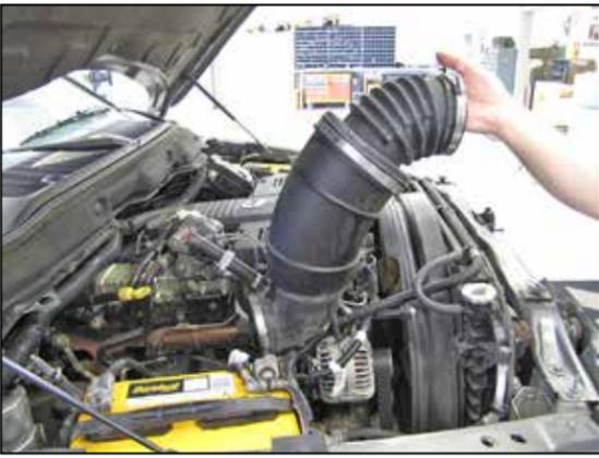
7. Loosen the hose clamp securing the factory intake hose to the turbo inlet and then disconnect the crank case vent hose from the pipe. Remove the complete intake hose from the vehicle as shown.
