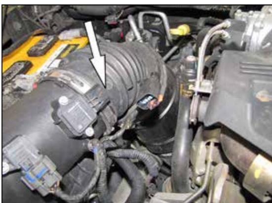
2. Release the locking tab and then disconnect the mass air sensor electrical connection.
