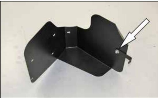
10. Install the heat shield mounting bracket (07158) onto the heat shield as shown using the provided hardware.
