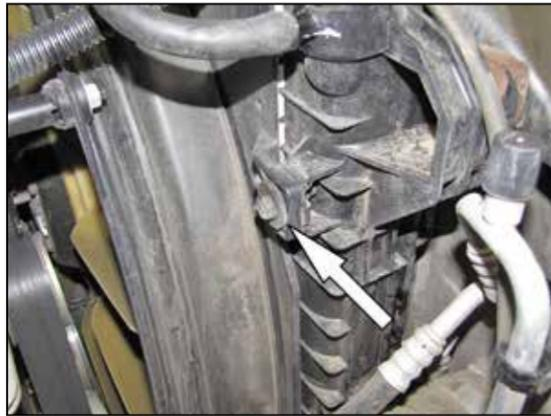
16. Remove the fan shroud bolt shown.
