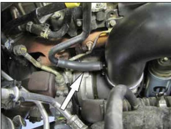
25. Install the provided crank case vent hose onto the fitting installed into the K&N® intake tube and then attach the open end to the factory vent pipe.
