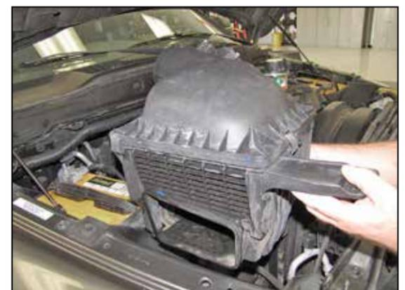
6. Remove the complete air box from the vehicle as shown.
