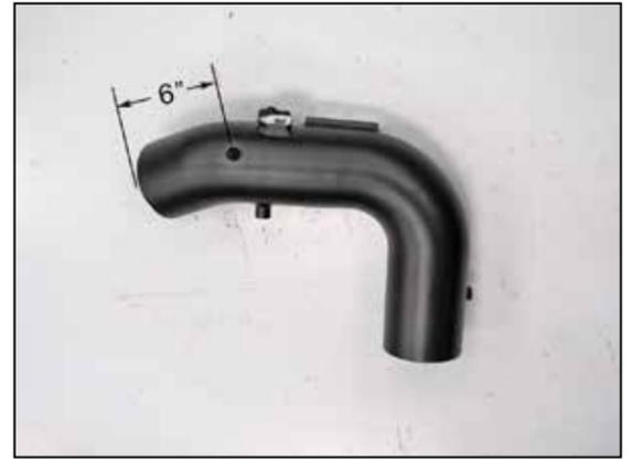
20. On vehicles equipped with a filter minder, drill a 5/8" id hole into the K&N® intake tube where shown.
