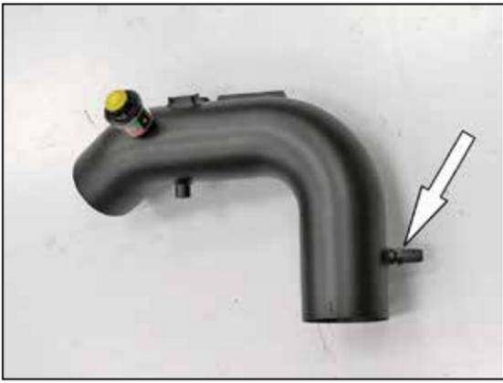
22. Install the 5/8 barbed, 1/4 npt crank case vent fitting provided into the K&N® intake tube as shown.
