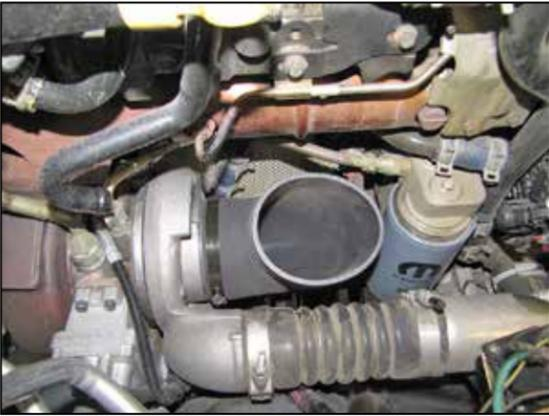
8. Install the K&N® elbow hose onto the turbo inlet and secure with the provided hose clamp.
