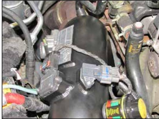
27. Reconnect the mass air sensor and inlet air temperature sensor electrical connections.
