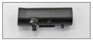
26. Install the mass air sensor assembly into the K&N® intake tube as shown and secure with the provided hardware.
