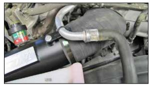
32. Secure the coolant pipe with the provided bracket (083166), mounting tie wrap and hardware to threaded stand-off on the K&N® intake tube.
