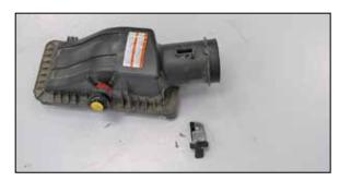
25. Remove the two screws securing the mass air sensor into the factory air box and then remove the sensor from the air box.
