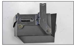
21. Install the factory air box mounting bracket onto the heat shield as shown so that the mount stand-offs installed in step #20 snap into the factory mounting grommets.
