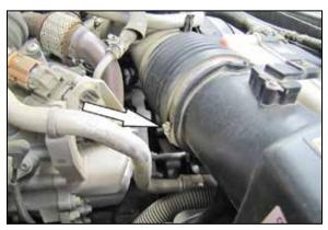
3. Loosen the hose clamp which secures the intake tube to the upper air box.
