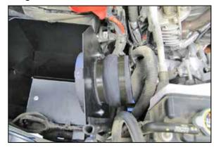
24. Install the silicone hump hose (08418) onto the filter adapter and secure with the provided hose clamp.
