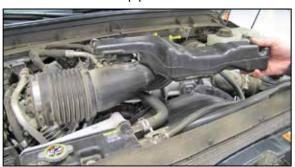
8. Loosen the hose clamp which secures the intake tube to the engine inlet then remove the intake tube from the vehicle.
