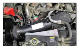
31. Install the K&N® intake tube into the silicone hose at turbo inlet, Align with the filter adapter and install the hump hose. Adjust the tube and hoses for best fit and then secure with the provided hose clamps.
