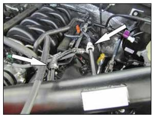
15. Connect the factory EVAP and Crank case vent lines to the fittings on the K8 N<sup>®</sup> intoke tube
