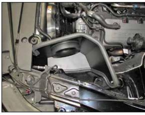
14. Set the heat shield onto the mounting bracket installed in step #9 and secure with the provided hardware.
