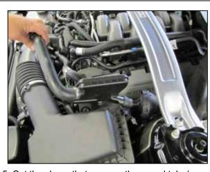
5. Cut the clamp that secures the sound tube/ chamber to the sound drum and then disconnect the sound tube/chamber from the sound drum.
