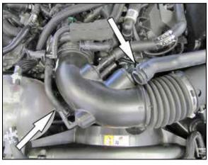
4. Depress the locking tabs and then disconnect the crank case vent hose and the EVAP vent hose. Then release the spring clamp and disconnect the sound tube from the intake tube.
