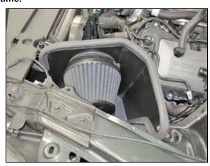
15. Install the K&N® air filter onto the adapter and secure with the provided hose clamp, then secure the heat shield and brackets to the air filter housing mounting location using the provided hardware.
