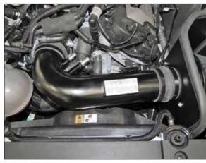
20. Install the K&N® intake tube into the hose at the filter adapter and then into the hose at the throttle body, adjust the tube and hoses for best fit and then secure with the provided hose clamps.
