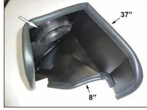
9. Install the provided edge trim onto the K&N® heat shield as shown. Install the air filter adapter into the heat shield and secure with the provided
