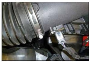
4. Disconnect the mass air sensor electrical connection.
