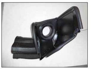
11. Install the provided fresh air duct into the heat shield as shown.
