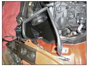
12. Install the heat shield assembly onto the inner fender and secure with the provided hardware. NOTE: The K&N<sup>®</sup> fresh air duct should be around the factory inlet duct.
