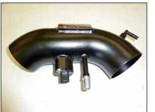
15. Install the Provided 90° fitting into the K&N® intake tube. Remove the mass air sensor from the factory housing and install it into the K&N® intake tube using the provided hardware.
