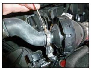
6. Release the one-time use clamp that secures the sound tube to the drum and then disconnect and remove the sound tube from the vehicle.
