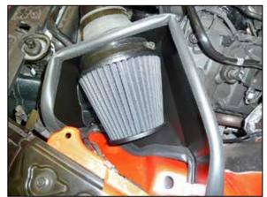
19. Install the K&N<sup>®</sup> air filter onto the filter adapter
