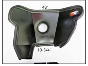
5. Disconnect the PCV hose from the passenger side lower intake tube, Remove the intake tube mounting bolt then loosen the hose clamp securing the intake tube to the turbo inlet and remove the tube from the vehicle. 11. Cut the 61"L edge trim to lengths of 10.75" and 48", install the edge trim onto the driver side heat shield as shown.
