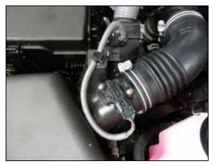
2. Disconnect the passenger and driver side mass air sensor electrical connection and unhook the harness's mounting clips.
