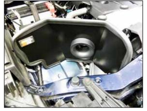
14. Install the passenger side heat shield assembly and secure with the provided hardware.
