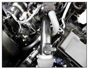
19. Install the driver side intake tube into the couplers, adjust the tube for best fit and then provided hose clamp cure with the
