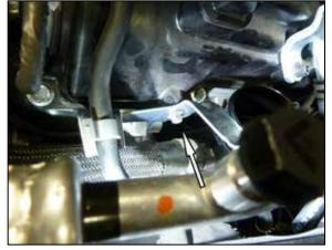
7. Remove the bolt that secures the driver side intake tube mounting bracket and then remove the bracket from the vehicle.
