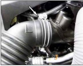
4. Loosen the hose clamps that secure the factory upper intake tubes to the turbo inlet manifolds and then remove the upper housings, intake tubes and filters.
