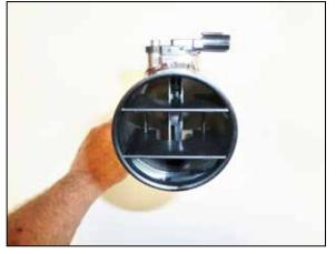
18. Install the air straighteners into the K&N intake tubes so that the blades are aligned as shown in relation to the mass air sensor.
