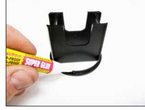
17. Apply four drops of the provided super glue to the air straighteners as shown.
