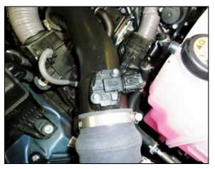
23. Reconnect the mass air sensor electrical connections.
