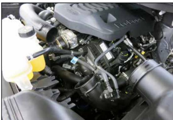
2. Loosen the three hose clamps that secure the factory intake tube to the turbo inlet tubes and air filter housing and then remove the intake tube from the vehicle.
