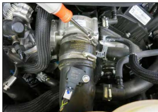
3. Loosen the hose clamp that secures the factory charge tube to the throttle body.
