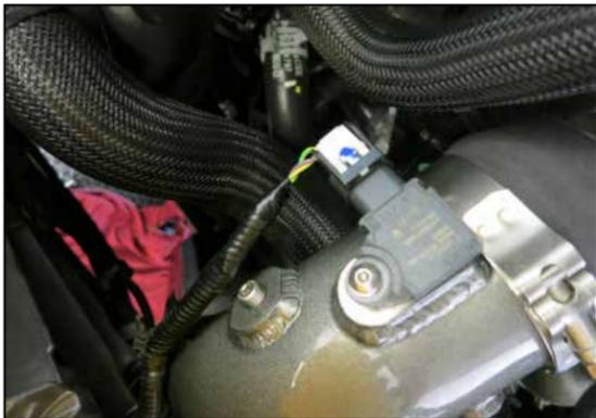
21. Reconnect the pressure sensor electrical connection.
