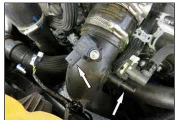
4. Disconnect the pressure sensor electrical connection. Disconnect the vent line quick disconnect fitting.
