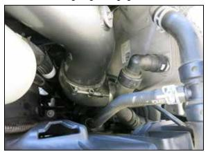
14. Adjust the tube and elbow coupler for best fit and then secure the hose clamps.
