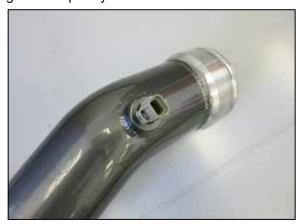
10. Remove the IAT sensor from the factory charge tube and install it into the K&N charge tube.
