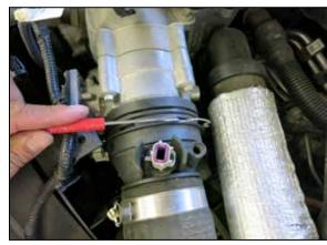
4. Using a small screwdriver or similar device, unlock the retaining clip that secures the factory charge tube quick connect coupler.
