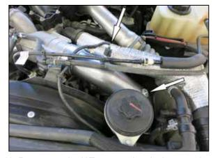
16. Reconnect the IAT sensor electrical connection and position the vent lines and harness.
