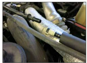
2. Disconnect the vent line at the quick connect
