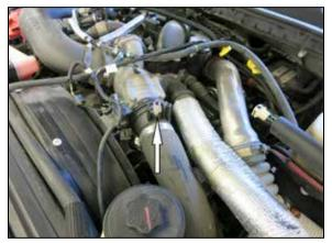
3. Disconnect the IAT sensor electrical connection and set the harness aside. Set the vent line aside for clearance while removing the factory charge tube.
