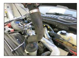
7. Separate the charge tube from the intercooler and then remove it from the vehicle.
