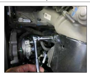
3. Remove the nut that secures the throttle body
