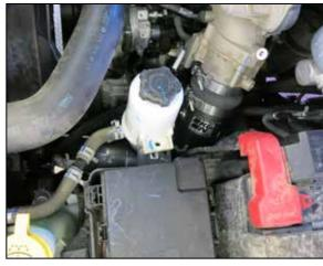
16. Secure the power steering reservoir with the factory bolt removed in step #9.
