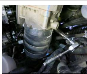
5. Loosen the hose clamp the secures the factory charge tube to the throttle body.
