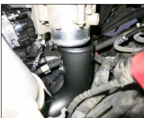
12. Feed the K&N intake tube down towards the intercooler and align with the throttle body.
