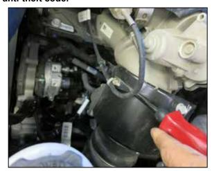
2. Separate the wiring harness from the cover over the throttle body.
