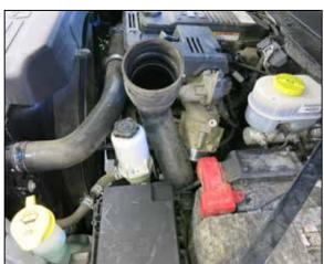
10. Remove the factory charge tube from the vehicle.
