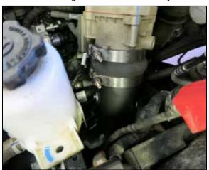
13. Install the provided hump hose and secure the charge tube to the throttle body with the provided hose clamps.
