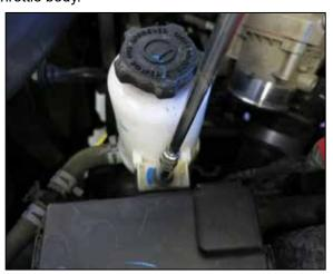
9. Remove the bolt that secures power steering reservoir. This will allow the reservoir to be moved to allow clearance for tube removal.
