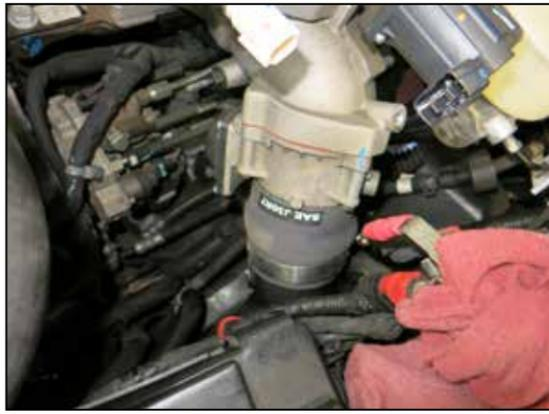
11. Install the provided hump coupler onto the charge tube with the clamps and then install on to the throttle body and secure with the hose clamps.
