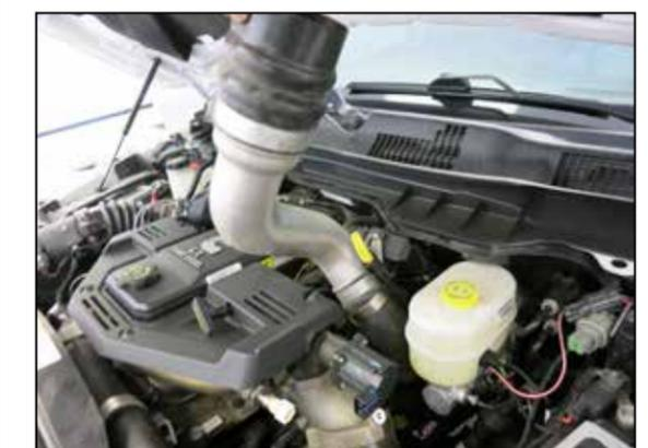
6. Guide the factory intercooler pipe up from between the throttle body and dip stick tube to remove it from the vehicle.
