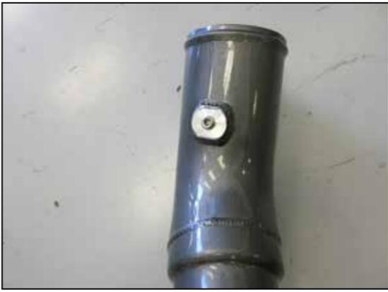
7. Install the provided 1/8" npt plug into the accessory part of the K&N charge tube. **NOTE: be sure to use pipe sealant on the threads of the plug.**
