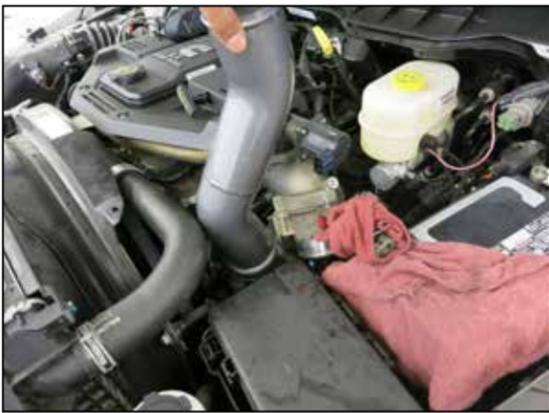
9. Route the K&N charge tube into position by passing the large side first down between the radiator hose and throttle body then back towards the rear of the engine compartment.
