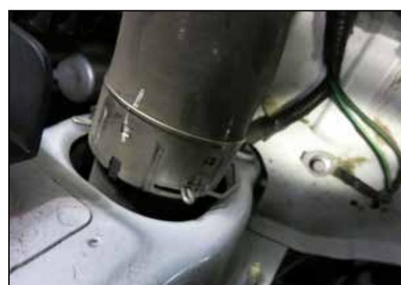
4. Release the charge pipe to intercooler quick connect fitting clip and lock it into the unlock position as shown.
