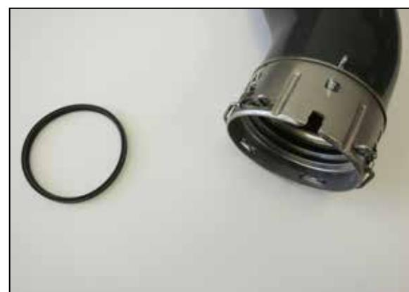
7. Carefully remove the factory O-Ring from the quick connect fitting. **NOTE: Be sure to note the direction of the lip on the seal.**
