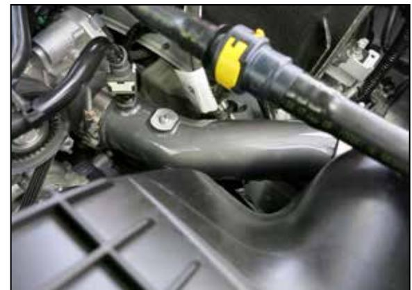
17. Connect the factory vent line to the quick connect fitting installed into the K&N charge tube and secure with the factory white locking clip.
