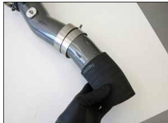
13. Install the clamps and angled coupler onto the K&N charge tube.
