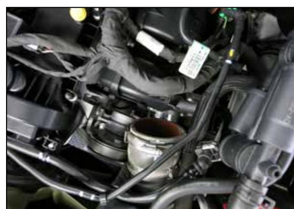
5. Disconnect the factory charge pipe from the throttle body and intercooler.
