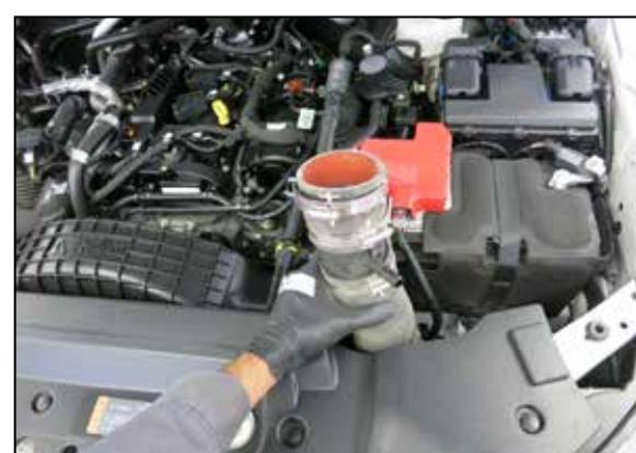
6. Remove the factory charge pipe from the vehicle.
