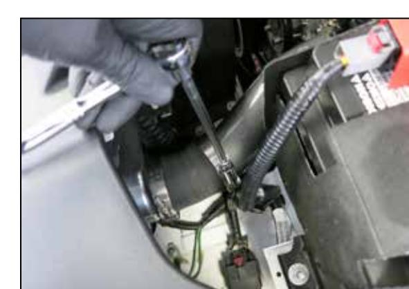
15. Connect the angle coupler onto the K&N intercooler quick connect fitting and slide the clamps into position.
