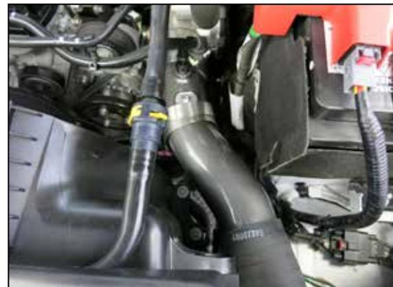
14. Set the K&N charge tube into position and align with the throttle body and intercooler connection.
