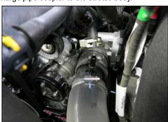
3. Release the white locking clip that secures the vent line quick connect fitting to the factory charge pipe and then disconnect the vent line from the charge pipe.
