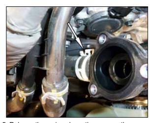
5. Release the spring clamp the secures the passenger side BOV hose to the charge tube and then disconnect the hose from the tube.
