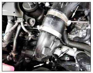
6. Remove the passenger side charge tube mounting bolt shown. Loosen the two hose clamps that secure the passenger side charge tube and then remove the charge tube from the vehicle.
