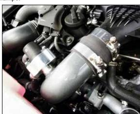
14. Install the passenger side K&N charge tube into the factory lower coupler, align with the upper hump coupler and install. Secure with the factory lower clamp and the upper hose clamp provided.
