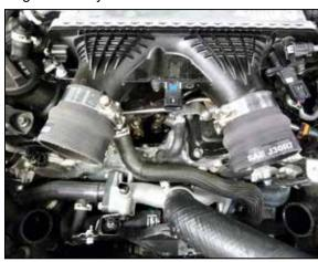
13. Install the provided hump couplers onto the intercooler and secure with the provided hose clamps.
