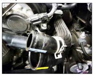
9. Release the clamp the secures the driver side BOV hose and then remove the hose from the vehicle.
