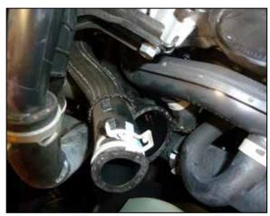
10. Release the clamp the secures the passenger side BOV hose and then remove the hose from the
