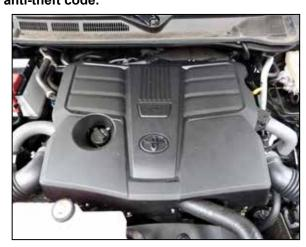
2. Pull up the engine cover along the front, then remove the engine cover from the vehicle.
