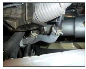
16. Rotate the heater hose spring clamps as shown to provide clearance for the BOV hose.
