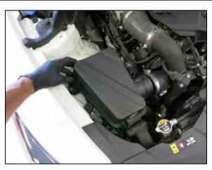
3. Loosen the three bolts that air filter housing to the inner fender and loosen the hose clamp that secures the intake tube to the air filter housing. Remove the air filter housing from the vehicle.
