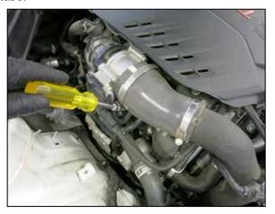
6. Loosen the hose clamp that secures the charge tube coupler to the throttle body.
