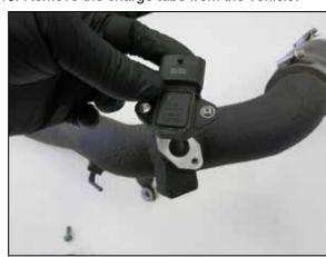
14. Remove the bolts that secure the pressure sensor to the charge tube and remove the sensor from the tube. **NOTE: These bolts will be reused.**
