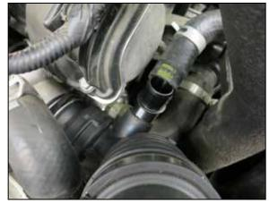
5. Release the spring clamp that secures the BOV hose to the intake tube and then disconnect the BOV hose. Now completely remove the intake tube.
