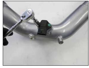
16. Install the factory pressure sensor into the K&N charge tube and secure with the factory bolts.
