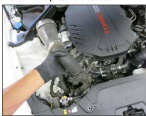
13. Remove the charge tube from the vehicle.
