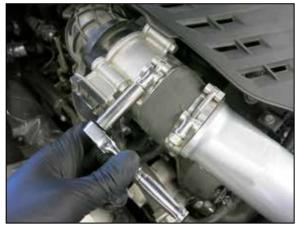
23. Check the charge tube positioning and then tighten all the hose clamps.
