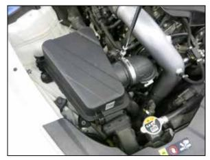
25. Reinstall the air filter housing and secure with the factory hardware and clamp.
