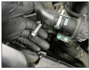
10. Remove the bolt that secures the charge tube to the engine.
