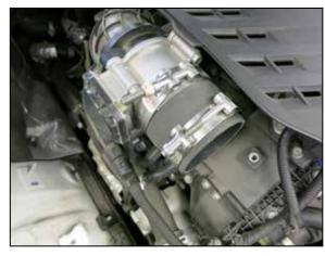
15. Install the provided coupler onto the throttle body and secure with the provided clamp.
