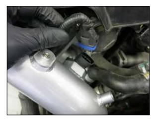
20. Reconnect the pressure sensor electrical connection.
