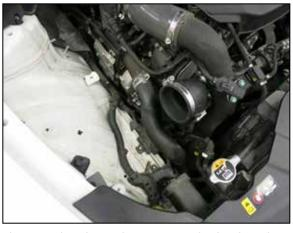
4. Loosen the clamp that secures the intake tube to the turbo inlet and then partially remove the intake tube from the vehicle.
