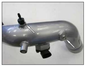
17. Install the provided 1/8npt pipe plug into the accessory port. Install the vacuum fitting into the K&N charge tube as shown. NOTE: this fitting uses 1/4npt threads, do not over tighten as the fitting may fracture. Some threads may be exposed once the fitting is properly installed.
