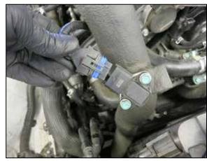
11. Disconnect the pressure sensor electrical connection.
