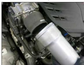
19. Install the K&N charge tube into the coupler at the throttle body and align for best fit.
