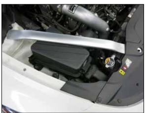
27. Reinstall the shock tower brace and secure with the factory hardware.
