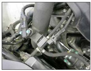
7. Disconnect the vacuum switch electrical connection.
