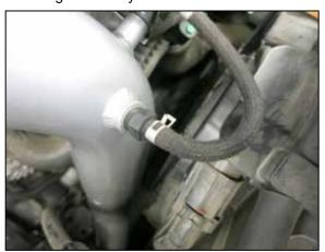
22. Connect the vacuum line to the fitting installed into the K&N charge tube.
