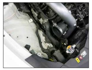
24. Reinstall the intake tube onto the turbo inlet.
