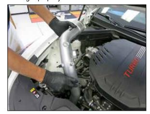
18. Install the K&N charge tube into the factory inter cooler coupler, do not tighten the clamp.
