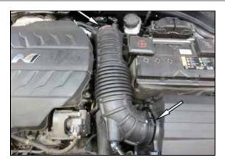
3. Loosen the hose clamps that secure the factory intake tube and then remove the intake tube from the vehicle.
