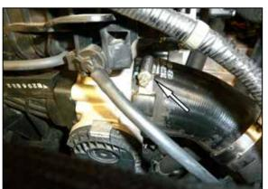
6. Loosen the hose clamp and spring clamps that secure the factory charge tube and then remove the charge assembly from the vehicle.
