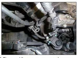
5. Disconnect the pressure sensor and vacuum switch electrical connection. Disconnect the vacuum line attached to the vacuum switch.
