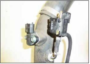
8. Remove the bolts securing the vacuum switch and pressure sensor and then remove the switch and sensor from the factory charge tube. The factory mounting bolts will be reused in a later step.
