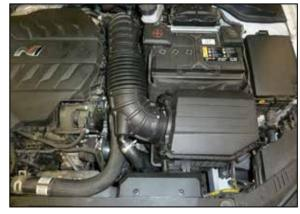
16. Reinstall the air filter housing and secure with the factory hardware. Reinstall the intake tube and secure with the factory clamps, reconnect the BOV and CCV vent hoses.
