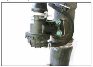
7. Disconnect the BOV vacuum hose from the charge tube and then remove the bolts securing the BOV and remove the valve from the tube. The factory bolts will be reused in a later step.
