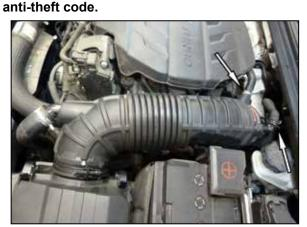
2. Release the spring clamps that secure the BOV and CCV hoses and then disconnect the hoses from the factory intake tube.
