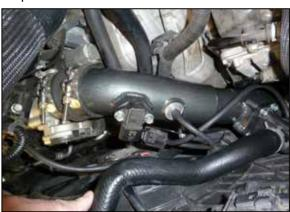
13. Install the K&N charge tube assembly so the lower coupler engages the intercooler. Align the upper section with the throttle body and slide the hump coupler into position. Adjust the tube for best fit and then tighten all the clamps.
