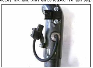
9. Install the provided NPT fitting and NPT plug into the K&N charge tube. Next attach the pressure sensor and vacuum switch to the charge tube using the factory mounting bolts. Install the provided vacuum hose onto the fitting and connect to the vacuum switch. Trim the vacuum hose for best fit.
