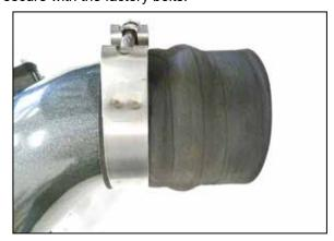
11. Install the hump coupler all the way onto the top of the charge tube. Do not secure the coupler.
