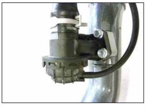
10. Install the BOV onto the Charge tube and secure with the factory bolts.
