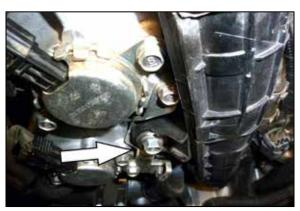
3. Remove the bolt that secures the charge tube to the engine.
