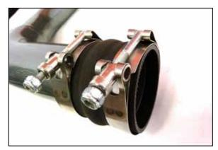
9. Install the provided hump coupler and clamps onto the K&N charge, slide the coupler all the way onto the tube.
