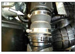
4. Loosen the hose clamp that secures the charge tube to the intercooler.
