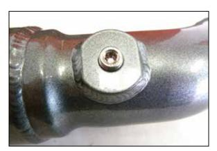
8. Install the NPT plug into the accessory port.
