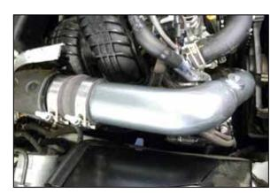
10. Install the K&N charge tube into the vehicle so the quick connect fitting engages the mating fitting, an audible click should be heard once the fitting is fully engaged. Slide the hump coupler into position and tighten the clamps.
