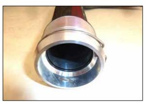
7. Remove the sealing O-ring and retaining clip from the factory charge tube and install them into the K&N charge tube.
