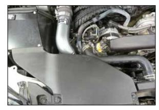
12. Reinstall the fresh air duct and clips.
