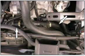
2. K&N intake system 69-8625TWR installed. Loosen the clamp on air box and lift up and remove the air box assembly. This will allow access to the charge tube.
