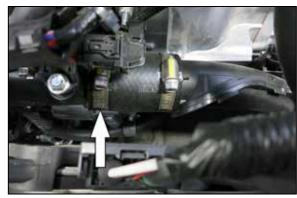
4. Loosen the hose clamp that secures the charge tube to the throttle body.
