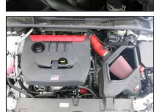
13. Reinstall the intake system. K&N intake system 69-8625TWR installed with Charge tube.
