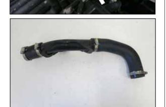
6. Separate the charge tube from the intercooler and throttle body and remove it from the vehicle.
