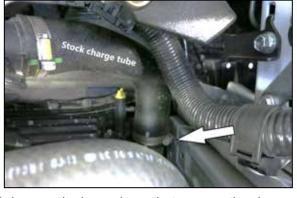
3. Loosen the hose clamp that secures the charge tube to the intercooler.
