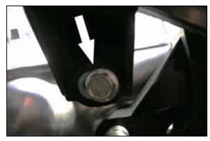
5. Remove the bolt that secures the charge tube to the transmission housing.
