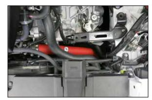
11. Position the charge tube and connect to the coupler on the intercooler and then connect to the throttle body, adjust for best fit and then secure with the hose clamps.
