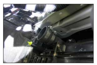
7. Install the provided step coupler onto the intercooler and secure with the provided hose clamp.
