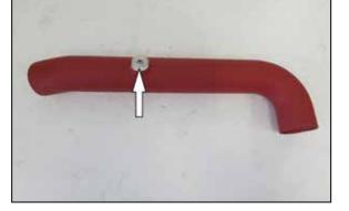
8. Install the provided NPT plug into the accessory port in the K&N charge tube.
