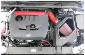
13. Reinstall the intake system. K&N intake system 69-8625TWR installed with Charge tube.
