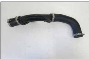
6. Separate the charge tube from the intercooler and throttle body and remove it from the vehicle.
