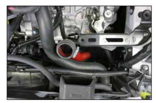
10. Feed the K&N charge tube down to the intercooler as shown.
