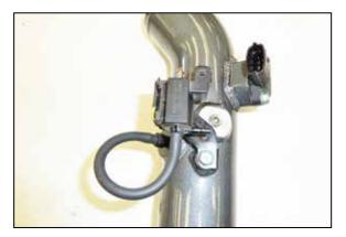
9. Install the provided NPT fitting and NPT plug into the K&N charge tube. Next attach the pressure sensor and vacuum switch to the charge tube using the factory mounting bolts. Install the provided vacuum hose onto the fitting and connect to the vacuum switch. Trim the vacuum hose for best fit.
