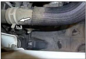
6. Loosen the hose clamp and spring clamps that secure the factory charge tube and then remove the charge assembly from the vehicle.
