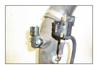
8. Remove the bolts securing the vacuum switch and pressure sensor and then remove the switch and sensor from the factory charge tube. The factory mounting bolts will be reused in a later step.
