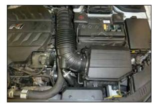
16.Reinstall the air filter housing and secure with the factory hardware. Reinstall the intake tube and secure with the factory clamps, reconnect the BOV and CCV vent hoses.
