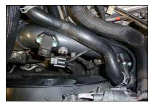
13. Install the K&N charge tube assembly so the lower coupler engages the intercooler. Align the upper section with the throttle body and slide the hump coupler into position. Adjust the tube for best fit and then tighten all the clamps.
