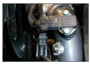
14. Reconnect the vacuum switch and pressure sensor electrical connections.
