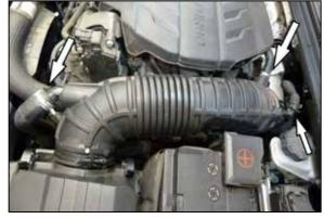
2. Release the spring clamps that secure the BOV and CCV hoses and then disconnect the hoses from the factory intake tube.
