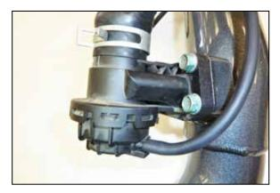
10.Install the BOV onto the Charge tube and secure with the factory bolts.
