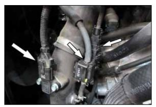
5. Disconnect the pressure sensor and vacuum switch electrical connection. Disconnect the vacuum line attached to the vacuum switch.
