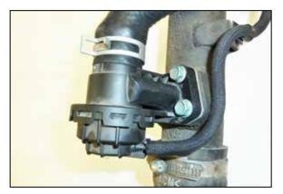
7. Disconnect the BOV vacuum hose from the charge tube and then remove the bolts securing the BOV and remove the valve from the tube. The factory bolts will be reused in a later step.
