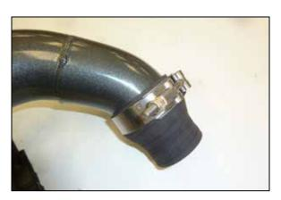
12. Install the step coupler onto the lower section of the charge tube and secure with the provided hose clamp.
