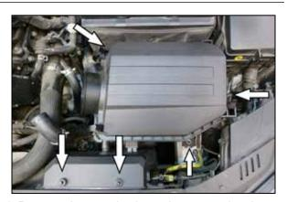
4. Remove the two plastic retainers securing the fresh air duct and then remove the three bolts that secure the factory air filter housing. Remove the factory air filter housing assembly from the vehicle.
