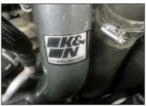
20. Install the provided decal onto the upper charge tube.
