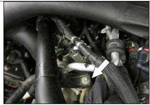
3. Reposition the coolant hose to gain access to the hot side charge tube mounting bolt and then remove the mounting bolt. Remove the hot side upper charge tube from the vehicle.
