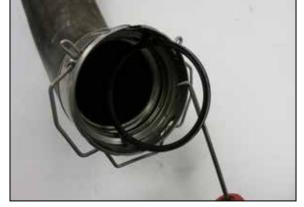
10. Remove the seal and retaining clip from the factory charge tube quick connect coupler to be used in the K&N quick connect coupler. NOTE: Pay close attention to the direction the seal is installed into the fitting.
