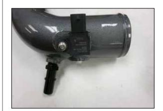
14. Remove the pressure sensor from the factory charge tube and install the sensor into the K&N charge tube using the provided bolt.
