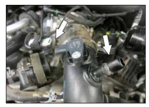
4. Disconnect the cold side charge tube pressure sensor electrical connection and then disconnect the CCV hose quick connect fitting.
