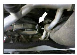
12. Install the provided rubber mounted stud into the charge tube mounting bracket.
