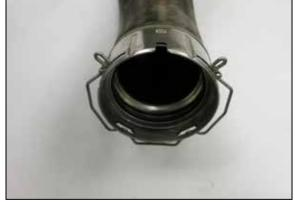
9. Pull the locking clip that secures the lower cold side charge tube to the intercooler. NOTE: Photo 1 shows charge tube connected to the intercooler, photo 2 shows the charge tube disconnected and the retaining clip in the unlocked position for reference. The charge tube is to be removed from under the vehicle.
