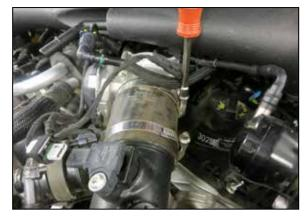
5. Loosen the hose clamp that secures the cold side charge tube to the throttle body and then loosen the clamp at the upper to lower charge tube connection.
