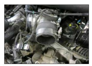
17. Install the remaining hump coupler onto the throttle body and secure with the provided clamps.
