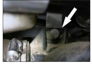
6. Remove the bolt that secures the lower part of cold side charge tube to the mounting bracket.
