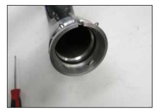
11. Install the seal and retaining clip into the K&N quick connect coupler. NOTE: Be sure to install the seal in the same direction as it was installed into the factory fitting.
