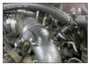
19. Reconnect the pressure sensor electrical connection and connect the CCV hose to the fitting installed into the K&N charge tube.
