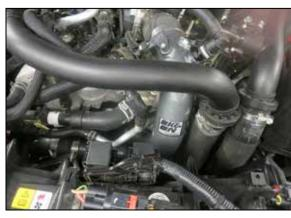
21. Reinstall the hot side upper charge tube and secure with the factory clamps.
