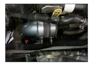
16. Install the provided hump coupler onto the lower charge tube and secure with the provided clamps.
