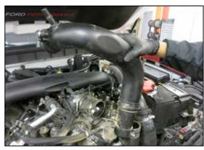
8. Remove the upper cold side charge tube from the vehicle.
