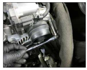
4. Remove the three bolts that secure the factory throttle body adapter to the throttle body and then remove the adapter.
