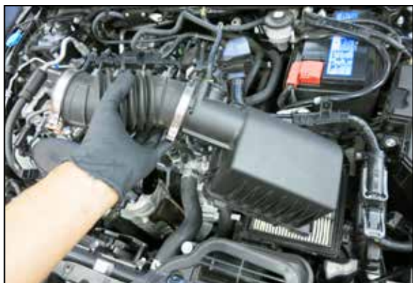
4. Release the upper air filter housing retaining clips and then remove the upper housing and intake tube.
