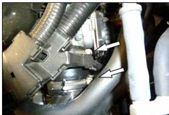
10. Loosen the charge tube coupler clamps and then remove the charge tube from the vehicle.
