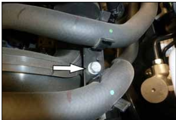
8. Remove the bolt that secures the hose holder to the charge tube then remove the holder from the vehicle.
