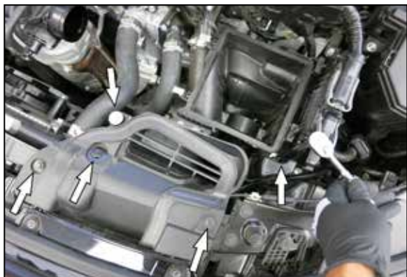
5. Remove the four bolts and one retaining clips that secure the lower air filter housing and fresh air duct, then remove the assembly from the vehicle.
