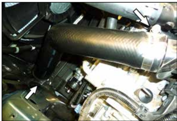
6. Loosen the hose clamps that secure the lower factory charge hose, then remove the charge hose.
