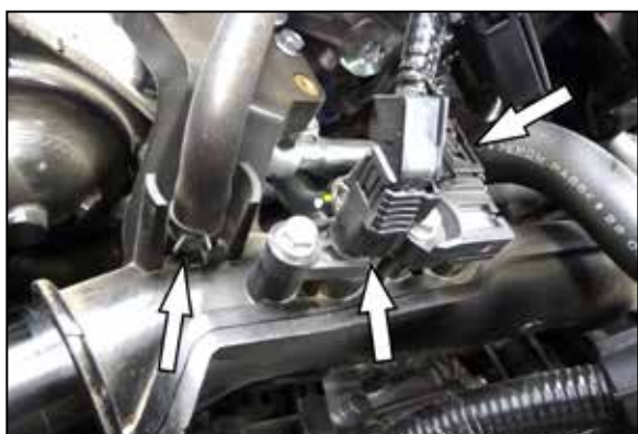
7. Disconnect the two pressure sensor electrical connections. Disconnect the vacuum hose from the upper charge tube.
