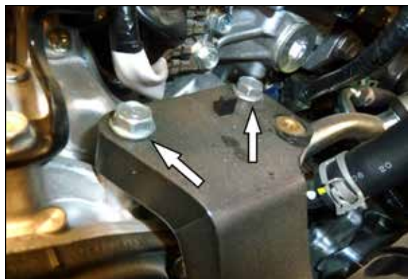
9. Remove the charge tube mounting bolts.
