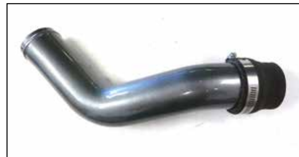
15. Install the step coupler onto the K&N lower charge tube and secure with the provided hose clamps.
