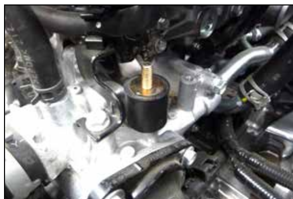
11. Install the provided rubber mounted stud onto the factory charge tube mounting location.
