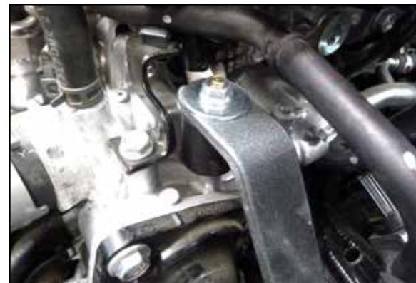
18. Secure the upper tube to the rubber mounted stud with the provided hardware.
