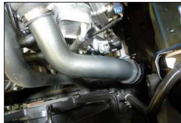
17. Install the lower charge tube, align both the upper charge tube and lower charge tube for best fit and then secure with the provided hose clamps.
