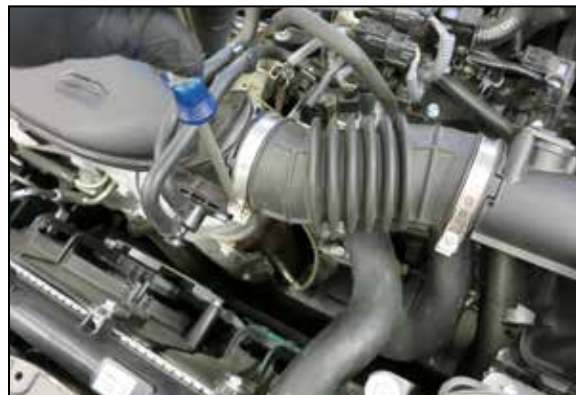
2. Loosen the hose clamp that secures the intake tube to the turbo inlet.
