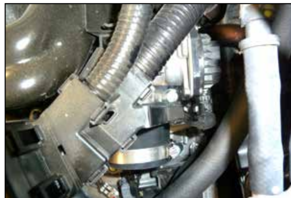
13. Install the provided straight coupler onto the throttle body and secure with the provide hose clamps.
