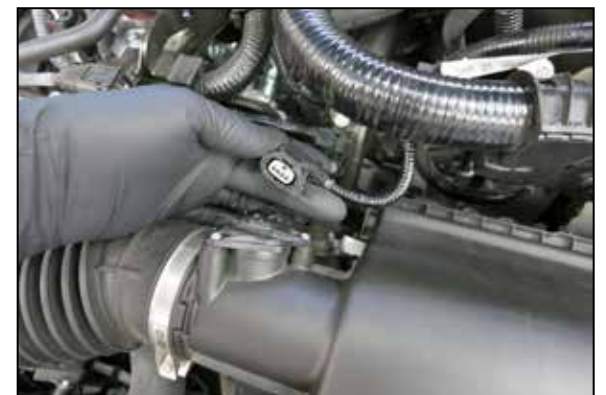
3. Disconnect the Mass Air Sensor electrical connection.
