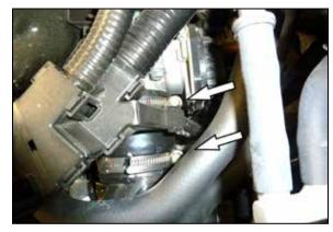
10. Loosen the charge tube coupler clamps and then remove the charge tube from the vehicle.
