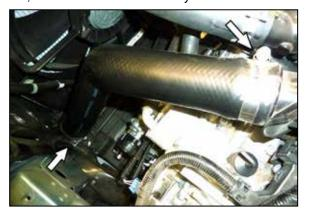
6. Loosen the hose clamps that secure the lower factory charge hose, then remove the charge hose.
