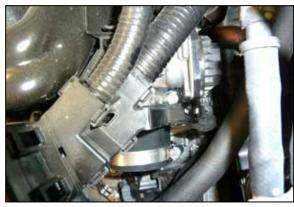
13. Install the provided straight coupler onto the throttle body and secure with the provide hose clamps.
