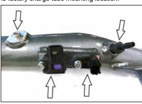
12. Remove the pressure sensors from the factory charge tube and install them into the K&N charge tube with the factory hardware. Install the 5/16" NPT barbed fitting and NPT plug into K&N intake tube as shown.
