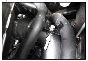
20. Install the factory hose holder onto the K&N charge tube and secure with the factory bolt.
