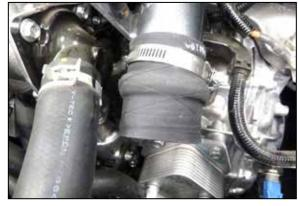
16. Install the provided step coupler onto the upper charge tube but do not secure.
