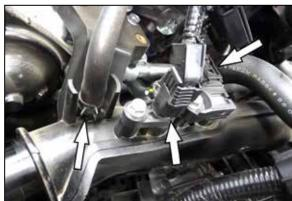
7. Disconnect the two pressure sensor electrical connections. Disconnect the vacuum hose from the upper charge tube.
