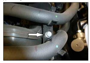
8. Remove the bolt that secures the hose holder to the charge tube then remove the holder from the vehicle.
