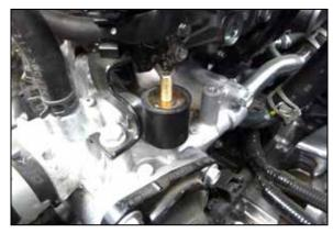
11. Install the provided rubber mounted stud onto the factory charge tube mounting location.
