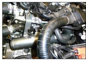
14. Install the K&N upper charge tube into the coupler at the throttle body and align the bracket to the rubber mounted stud.
