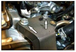
9. Remove the charge tube mounting bolts.
