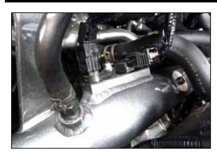
19. Connect the vacuum line to the npt fitting installed into the upper charge tube then reconnect the pressure sensor electrical connection.
