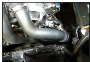
17. Install the lower charge tube, align both the upper charge tube and lower charge tube for best fit and then secure with the provided hose clamps.
