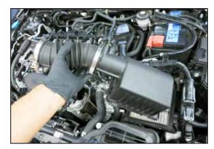
4. Release the upper air filter housing retaining clips and then remove the upper housing and intake tube.
